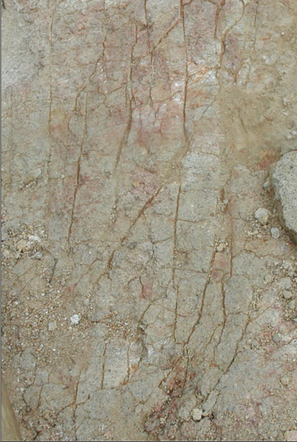
Plate 15 - Detail of Fractures Forming an Orthogonal Pattern on the Floor of Landslide B (Photograph taken on 12 October 2000)
