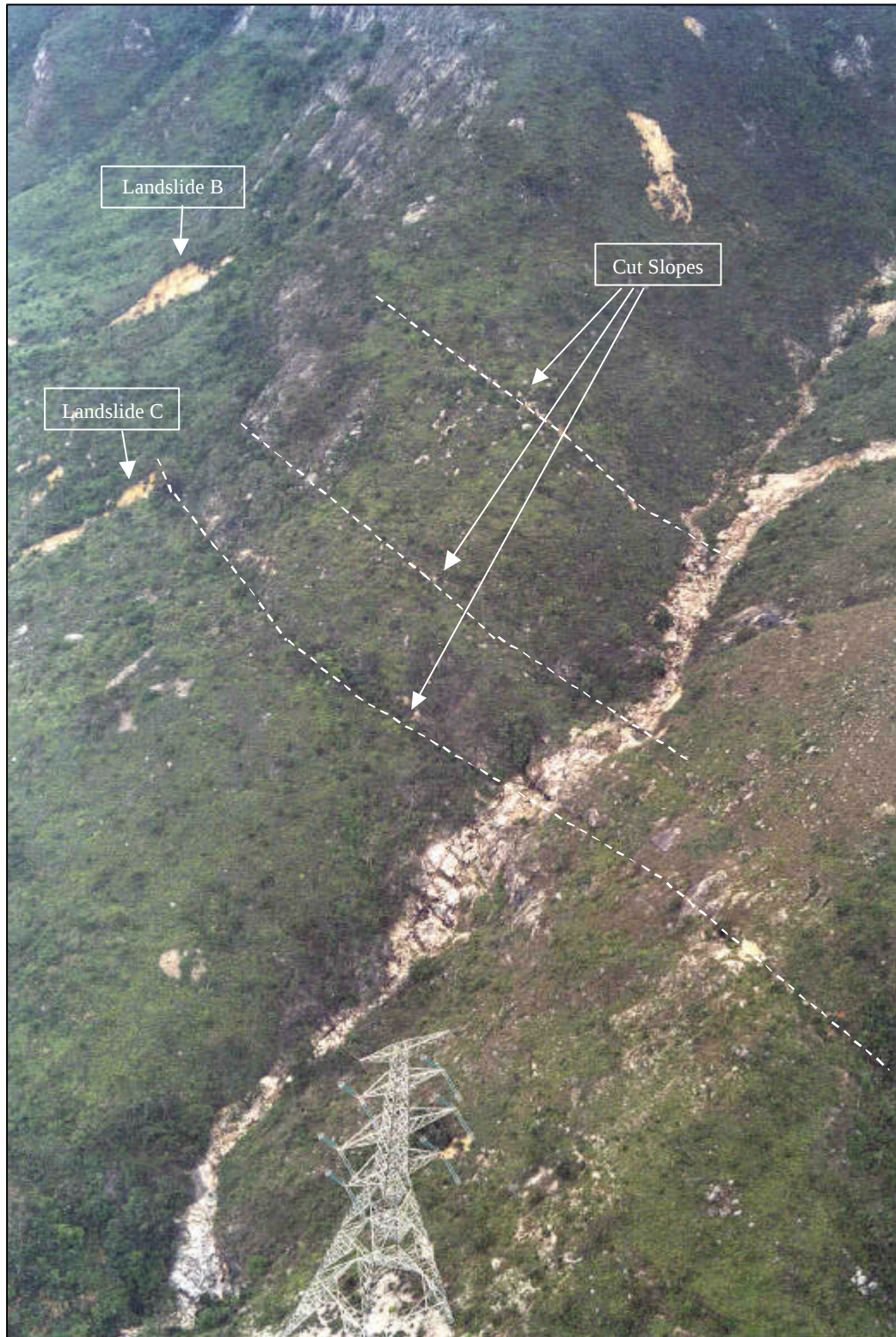
Plate 42 - Oblique Aerial View Showing the Cut Slopes Formed During the Mining Works before 1945 (Photograph taken on 30 June 2000)
