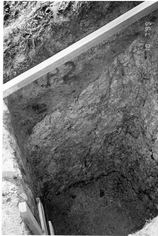
Plate 21 – Trial Pit TP2: Western Face of Pit Exposing Fill Overlying Insitu Ground Profile (Photograph Taken on 7 October 1999)
