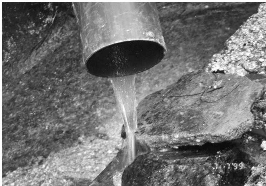
Plate 14 – Discharge of Water from Scar (Plate 13) through PVC Collection Pipe Providing Indication of Flow (Photograph Taken on 7 July 1999)
