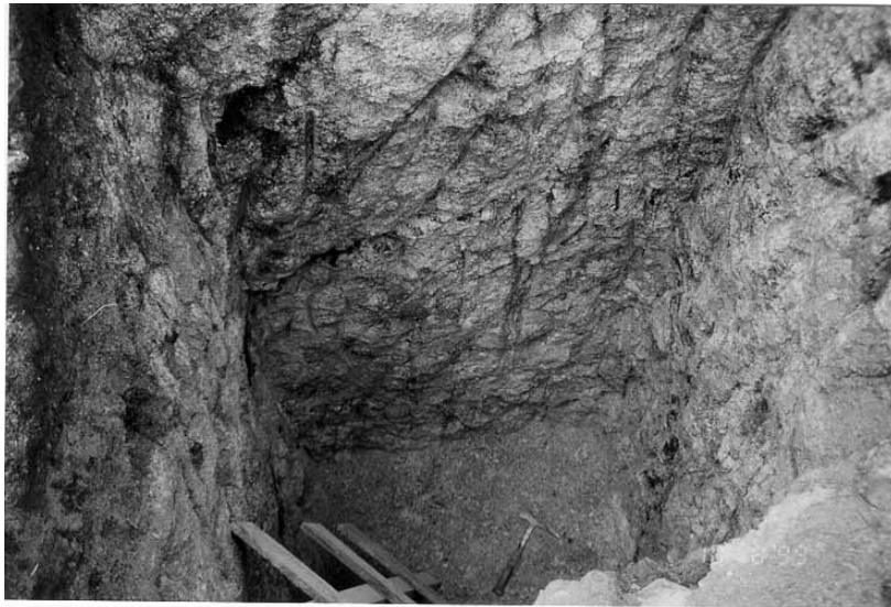
Plate 20 – Trial Pit TP1: Grade IV/V Weathering Profile Exposed in Pit. Note Staining on Relic Joints and Dark Brown/Black Manganese Oxide Deposits (Photograph Taken on 8 October 1999)
