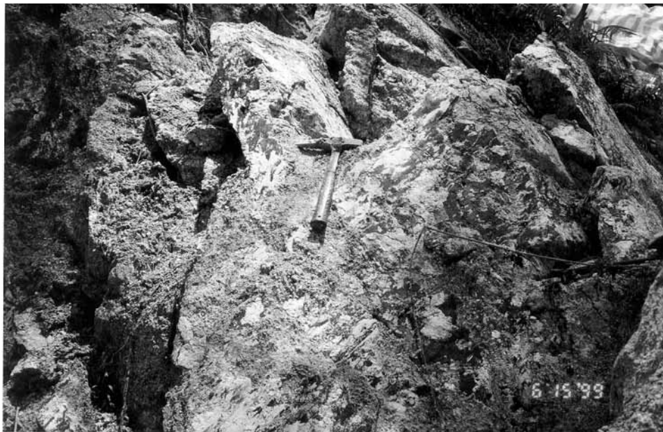
Plate 28 – Manganese Oxide (Black) Infill on Relic Joint Surfaces Exposed in Landslide Debris. Infill Thickness up to 2 mm (Photograph Taken on 15 June 1999)
