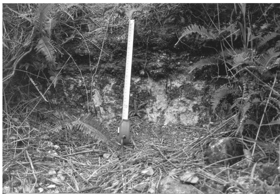
Plate 13 – View of the Discoloured and Vegetated Main Scarp of MS2 (Photograph Taken on 30 August 1999)
