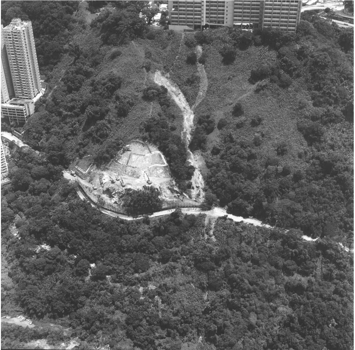
Plate 1 – Oblique View of the Landslide Site Indicating Convergent Debris Trails and Subsequent Runout to Victoria Road. VTC Pokfulam Skills Centre Visible in Upper Portion of Frame. Upper Baguio Villas (Block 26) and Lower Baguio Villas (Block 44) Separated by Victoria Road Visible on Left of Frame. Slope Works in Progress above Victoria Road Associated with Victoria Road Improvement Stage 2 Phase II Project (Photograph Taken on 2 September 1999)
