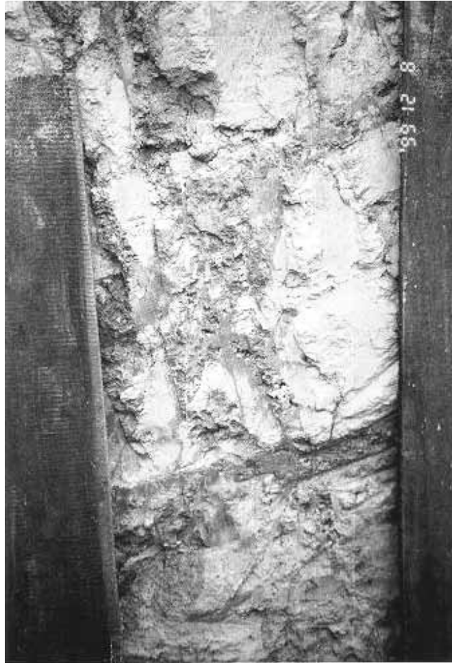
Plate 21 – Trial Pit TP2: General View Indicating Open, Blocky Structure of Grade IV Tuff (Photograph Taken on 8 December 1999)
