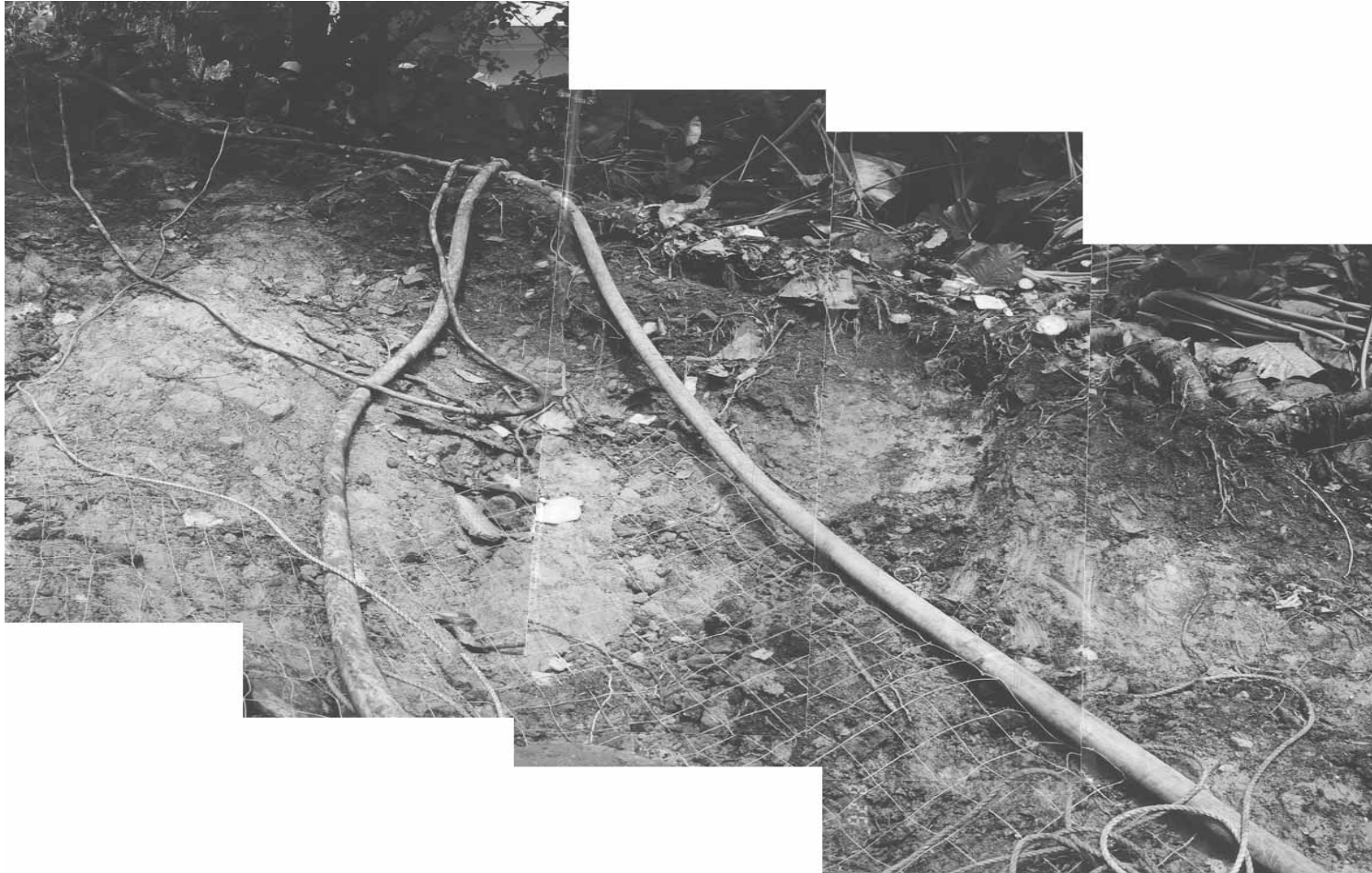
Plate 7 – View East across Southern Flank of Landslide A. Note Shallow Depth of Fill and Planar Exposure of Natural Ground in Scar. Note also Refuse Content of Fill (Photograph Taken on 26 August 1999)
