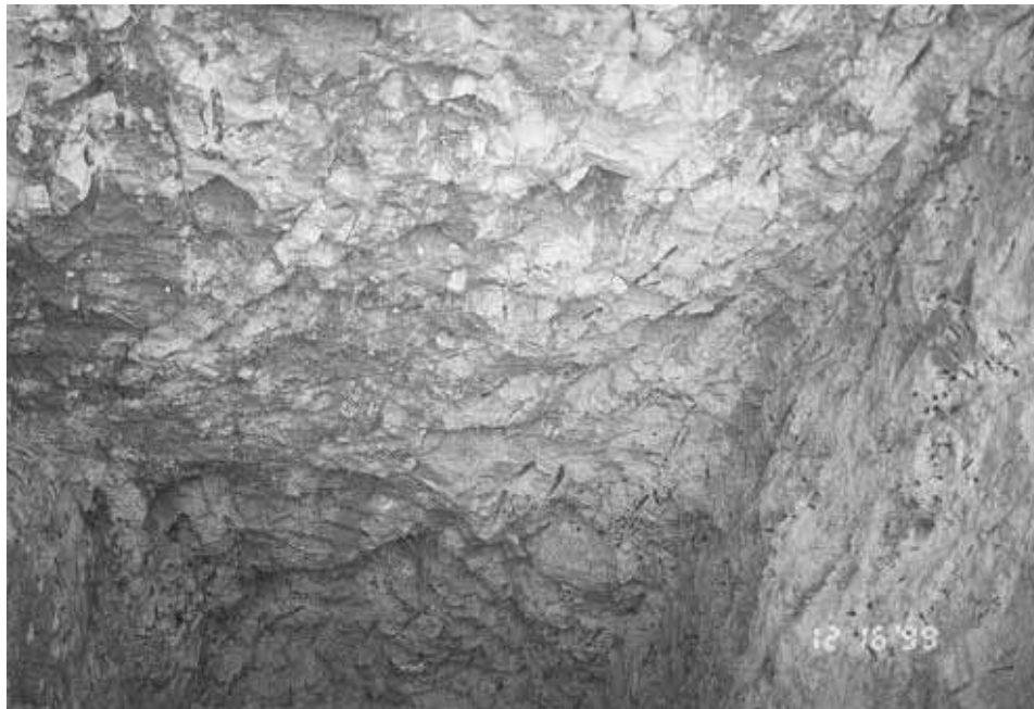
Plate 23 – Trial Pit TP5: General View of Pit Showing Exposure of Grades IV and V Tuff (Photograph Taken on 16 December 1999)
