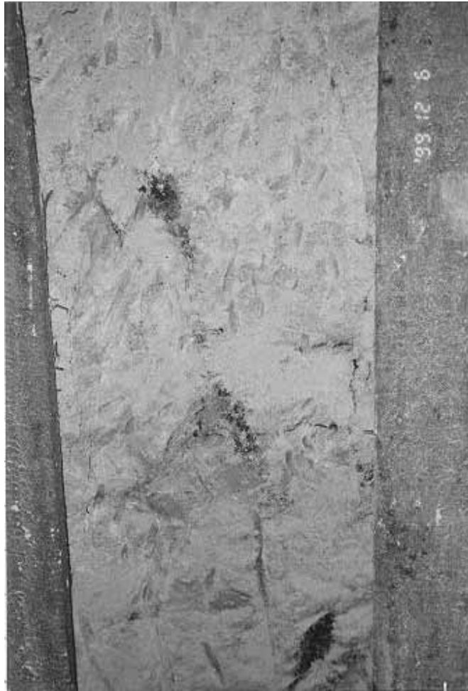
Plate 18 – Trial Pit TP1: General View Showing Insitu Weathering Profile of Fine Ash Vitric Tuff (Photograph Taken on 6 December 1999)
