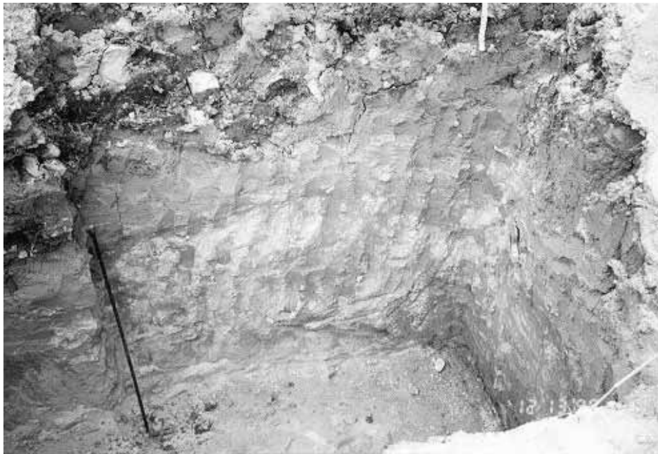
Plate 26 – Trial Pit TP8: General View of Pit Showing Exposure of Grades IV and V Tuff. Note Landslide Debris Remaining beneath Shotcrete at Top of Frame (Photograph Taken on 13 December 1999)
