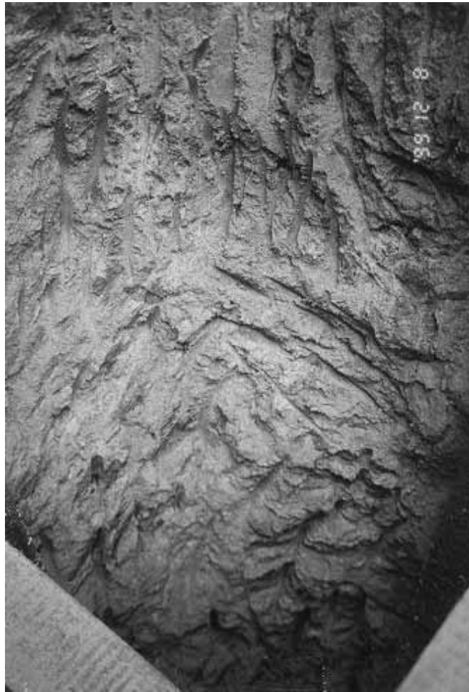
Plate 19 – Trial Pit TP2: General View Showing Insitu Weathering Profile of Fine Ash Vitric Tuff (Photograph Taken on 8 December 1999)
