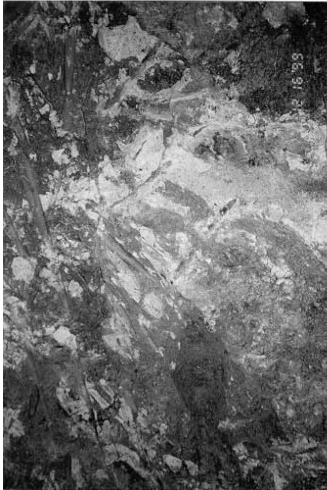
Plate 27 – Trial Pit TP5: Exposure of Grade III/IV Tuff in Western Face of Pit. (Photograph Taken on 16 December 1999)
