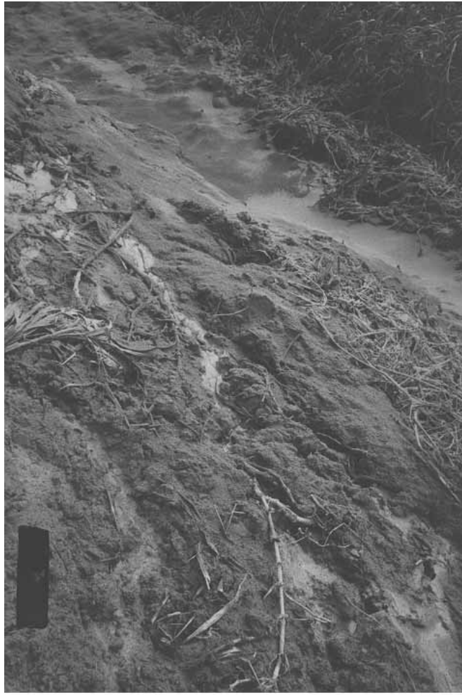
Plate 15 – Erosion Channels within Landslide Scar downslope of Point of Confluence (Photograph Taken on 26 August 1999)
