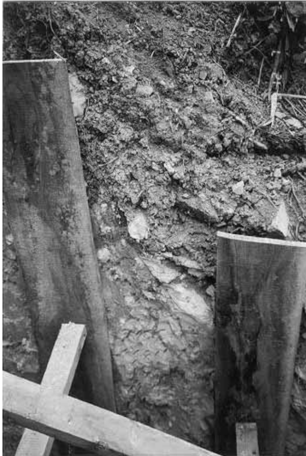
Plate 20 – Trial Pit TP3: South-East Face of Pit Exposing Fill Overlying Insitu Profile (Photograph Taken on 7 December 1999)
