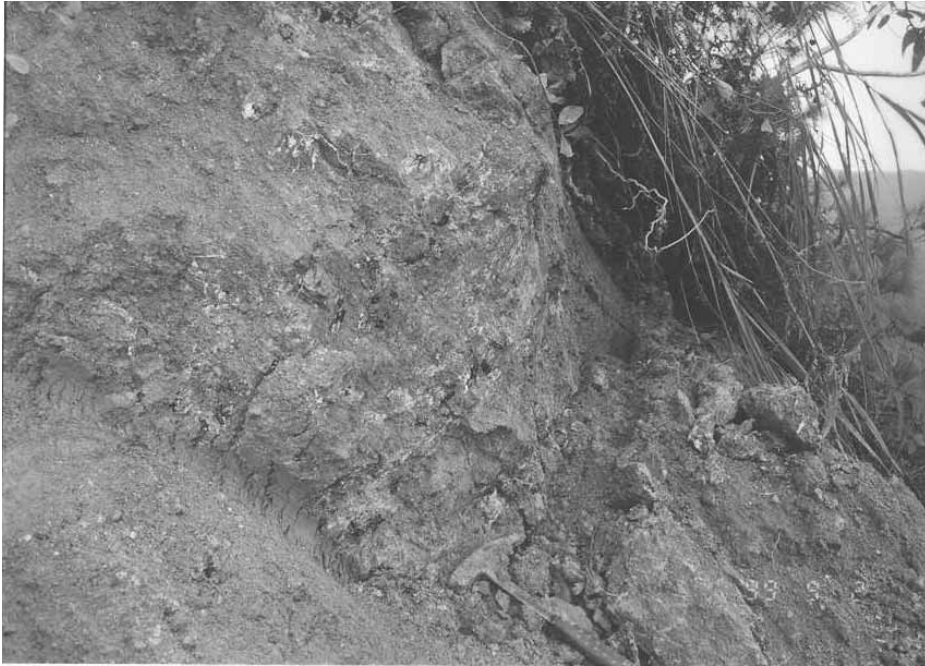
Plate 14a – CDT with Closely-Spaced Discontinuities along Western Flank of the Scar (Photograph Taken on 2 September 1999. See Figure 11 for Location)
