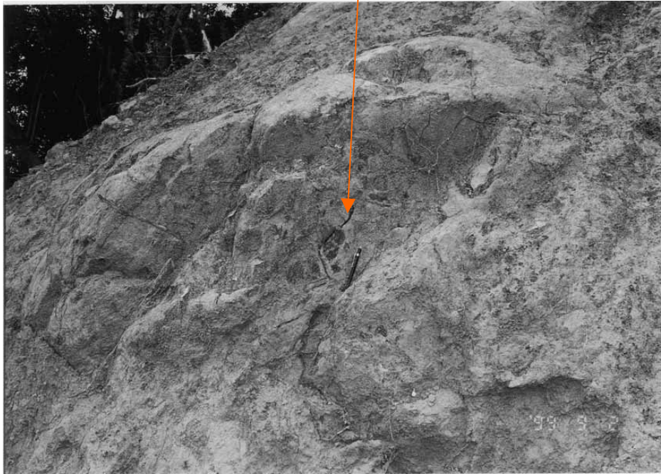
Plate 12a – MDT Corestone within CDT (Surface of CDT is Covered with Previous Tension Crack/Joint Infilling Material). Note Slickensided Manganese Oxide Stained Release Planes. (Photograph Taken on 2 September 1999. See Figure 11 for Location)
