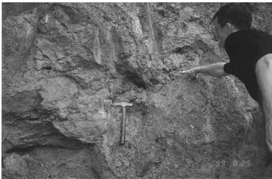
Plate 30 - Concentration of Termite Galleries/Erosion Pipes along Interface of Grade V Material with Underlying Corestone (Bedrock?) in Central Portion of Main Scarp (Photograph Taken on 29 August 1999)
