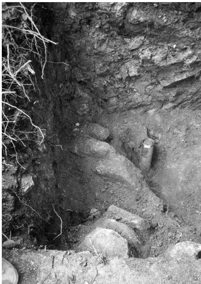
Plate 19 - Grade III/IV Quartz Syenite Exposed in Trial Pit TP2 with Closely to Very Closely Spaced, Saprolite Infilled Joints (Possible Tension Features) (Photograph Taken on 29 October 1999)
