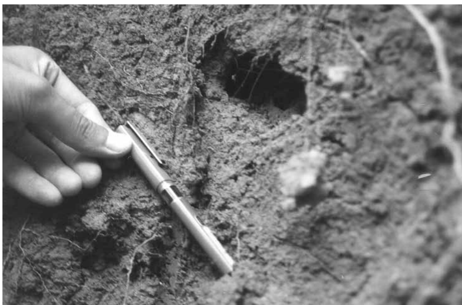
Plate 31 - Example of Termite Gallery/Erosion Pipe Exposed in Grade V Quartz Syenite (Photograph Taken on 29 October 1999)
