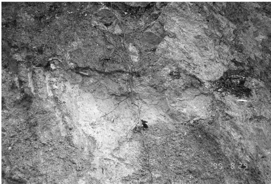
Plate 17 - Close-up of Clay Infilled Joint Exposed in Main Scarp (Photograph Taken on 29 August 1999)
