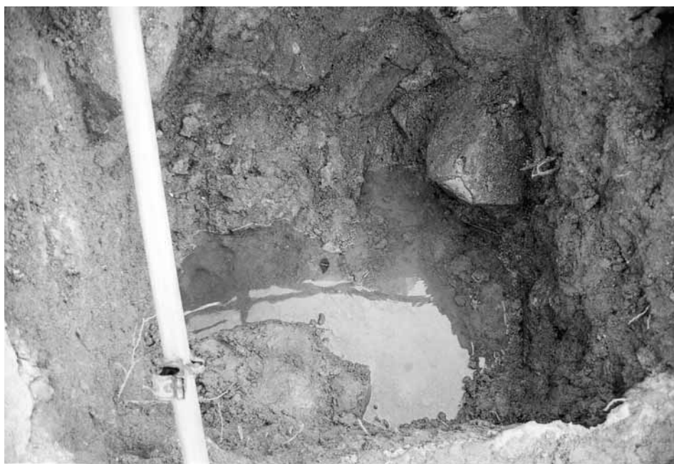
Plate 33 - Trial Pit TP4: Seepage Ponding in Base of Pit (Photograph Taken on 29 October 1999)
