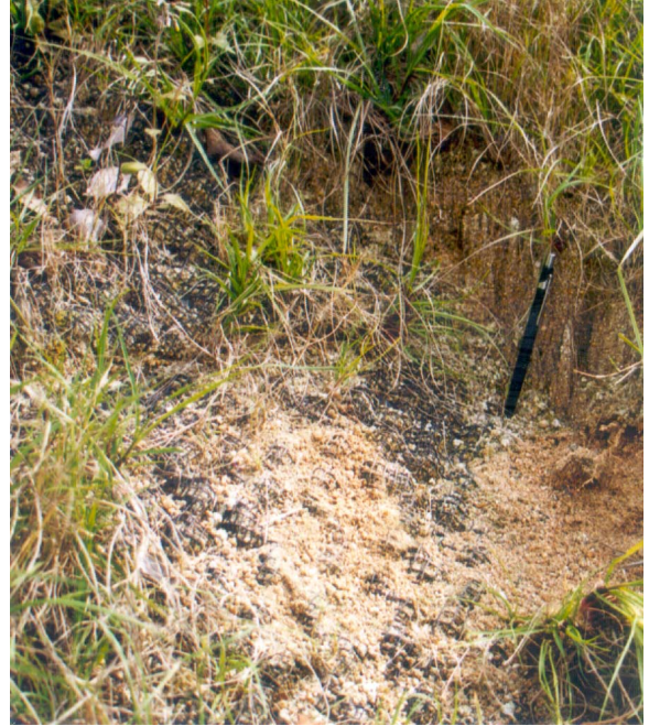
(b) Erosion of soil placed above erosion control mat on 45° soil slope
