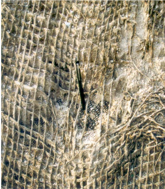
(e) Erosion of soil surface through biodegradable erosion control mat
