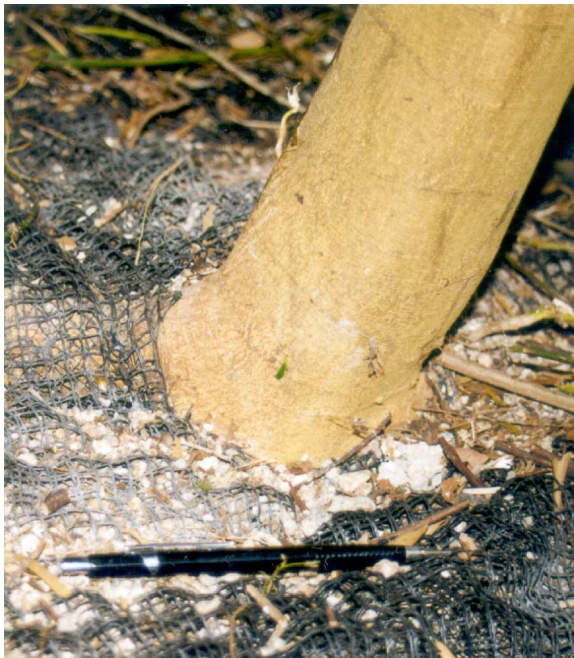
(c) Potential strangulation at base of stem of large plants by erosion control mat
