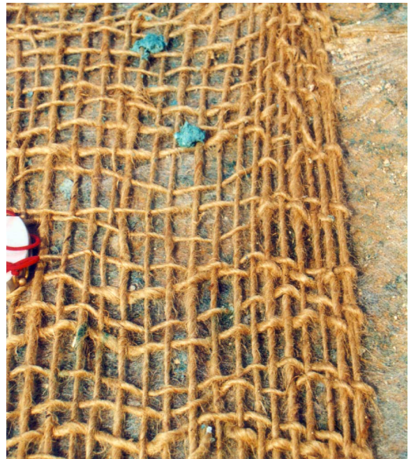
(d) Close-up view of biodegradable erosion control mat (Soil Saver)
