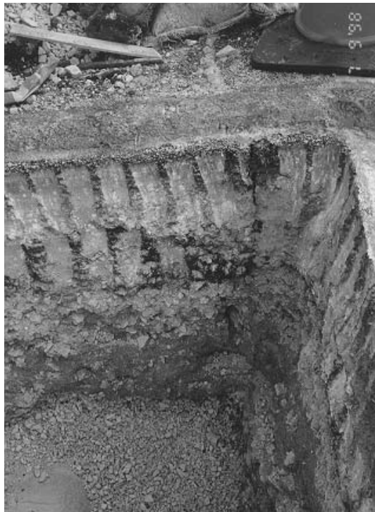
Plate 39 – Close-Up of Cracking Extending Vertically Beyond Base of Trial Pit ATP1. (Photograph Taken on 9 July 1998)
