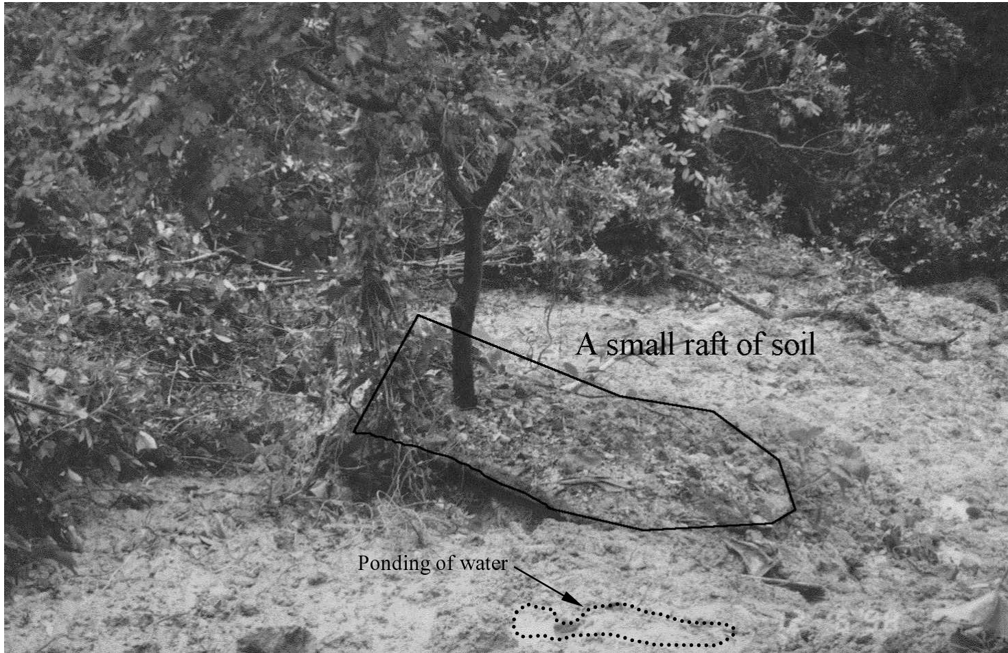
Plate 5 - A small Raft of Soil near Slope Crest (Photograph taken on 12 June 1998. See Figure 4 for Location of Photograph)
