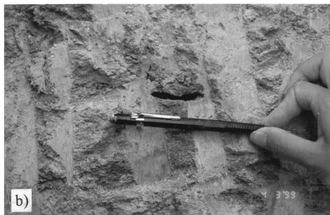
Plate 28 – Close-up Views of Voids/Soil Pipes Exposed in Trial Trench TT1 (Photographs taken on 4 March 1999 - see Plate 27 for locations)
