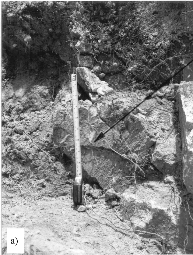
Plate 33 – Views Showing Infilling to Joints/Cracks within H-MDT (Photographs taken on 23 March 1999)
