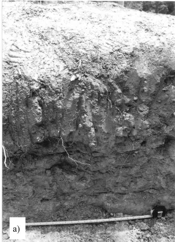
Plate 31 – Views of Face C, Trial Pit TP7 Showing Lateral Cracking/Voiding within CDT (Photographs taken on 4 March 1999)
