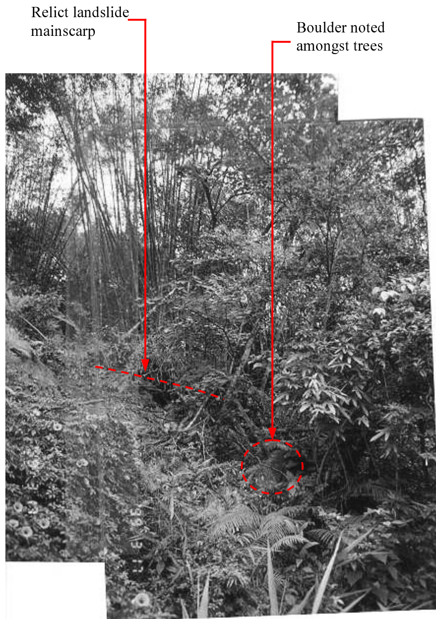
Plate 10 – The "Stable" Portion of the Main Southwest-facing Slope of the Feature between Landslides Nos. 2 and 3. The Boulder is considered indicative of Previous Instability within this part of the Slope (Photographs taken on 17 March 1999)
