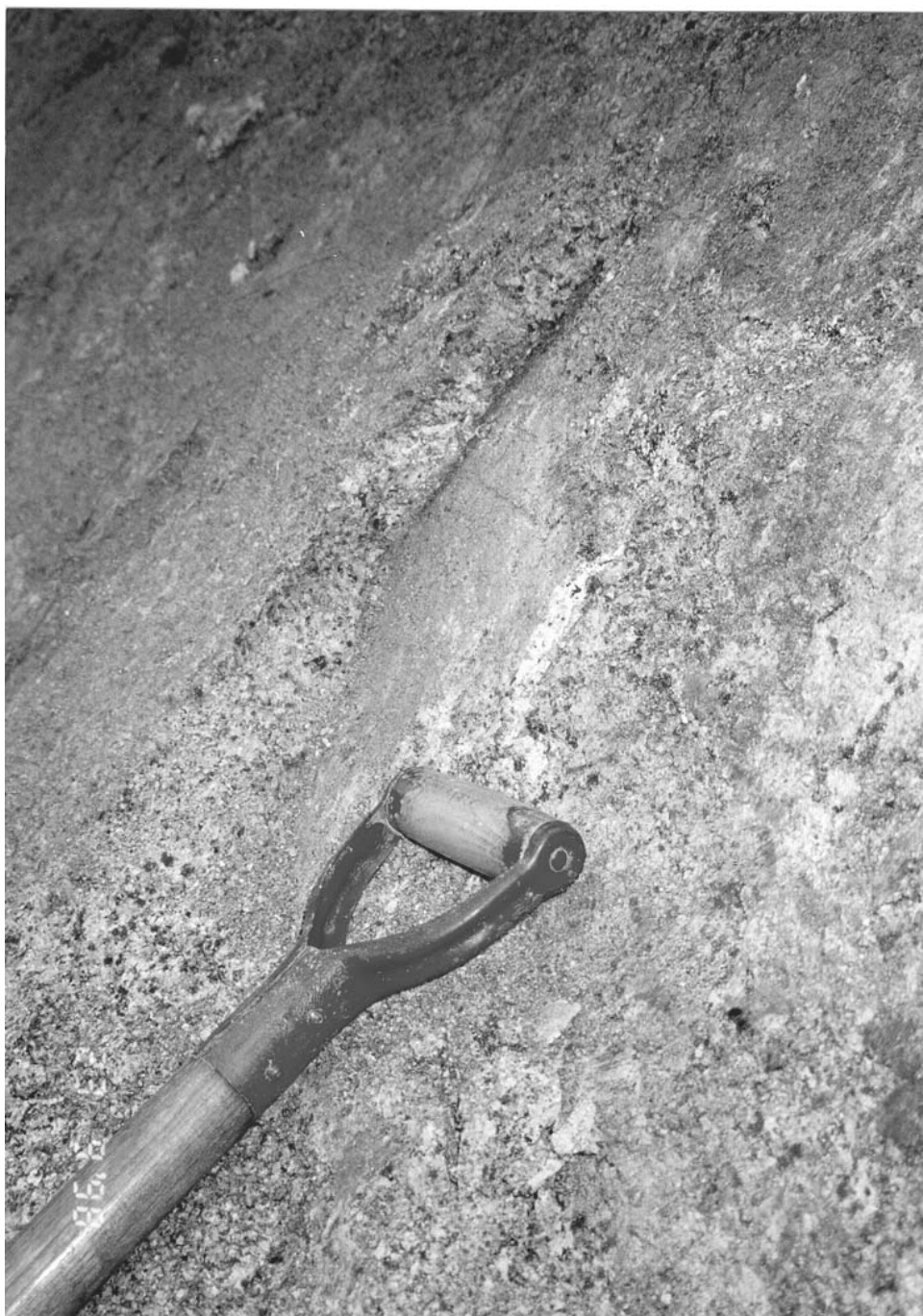
Plate 6 – View of Kaolin Infilling along the Eastern Failure Plane (Photograph taken on 23 September 1998)
