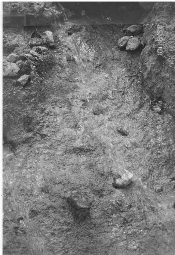
Plate 10 – Close-Up of Exposed Insitu Material in Landslide Scar. Note Water (From PVC Pipe - Plate 7) Flowing Across Exposure. (Photograph Taken on 10 June 1998)
