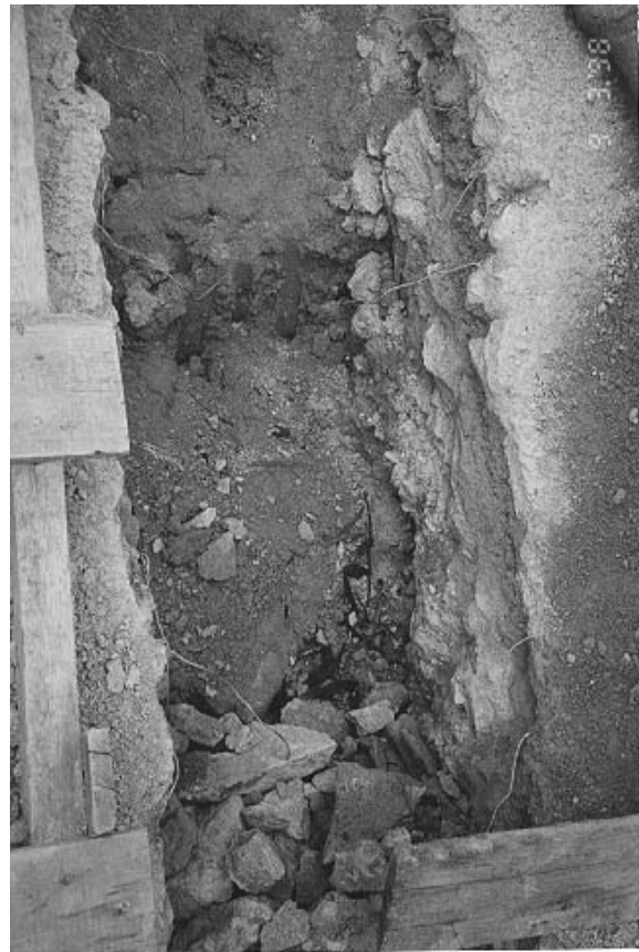
Plate 45 – Strip S1 Showing Fill Exposed Beneath Hard Surfacing 2 m Below Crest. Note Numerous Layers of Surfacing (Photograph Taken on 3 September 1998)
