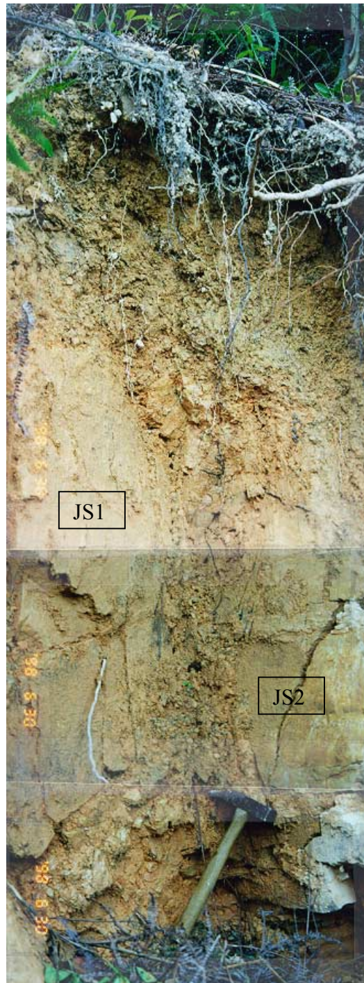
Plate 18 – Dominant West to West-Northwest (JS1) and North-Northeast (JS2) dipping Joint Sets in the Upper Landslide Backscarp (Photographs taken on 30 June 1998)
