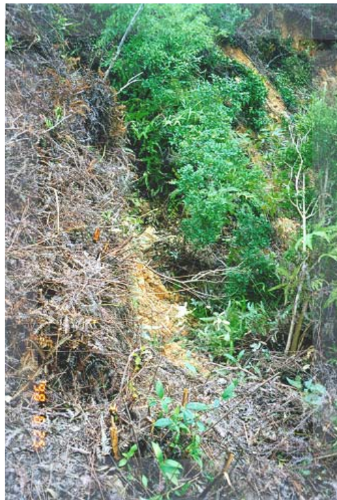
Plate 11 – Remnants of Tension Cracking in the Northern Portion of the Upper Landslide Backscarp (Photographs taken on 25 June 1998)
