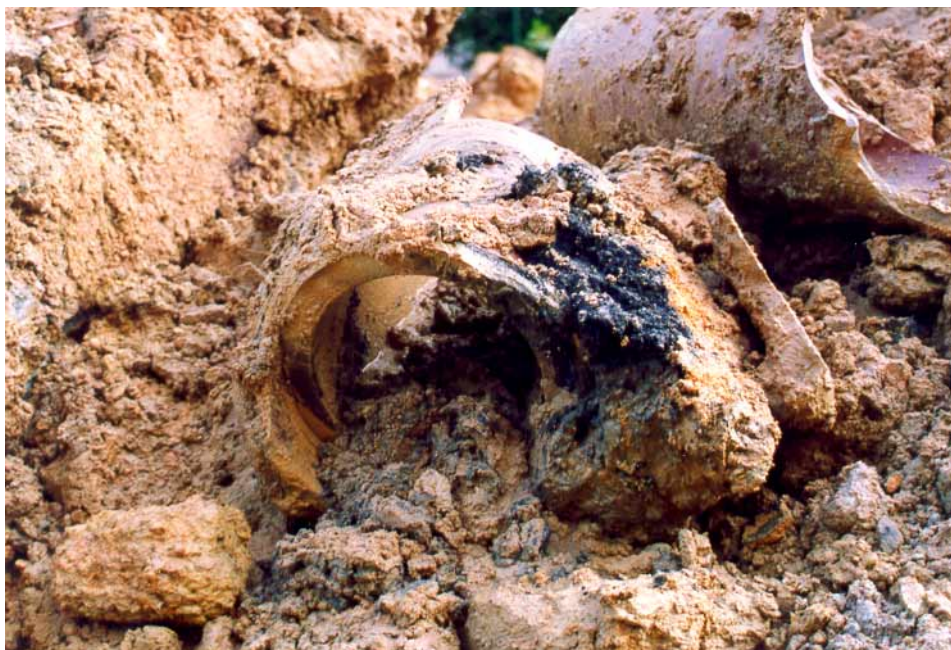
Plate M10 - Broken Section of the Foulwater Sewer with Black-stained Soil Recovered from the Landslide Debris (Photograph taken on 27 July 1994)
