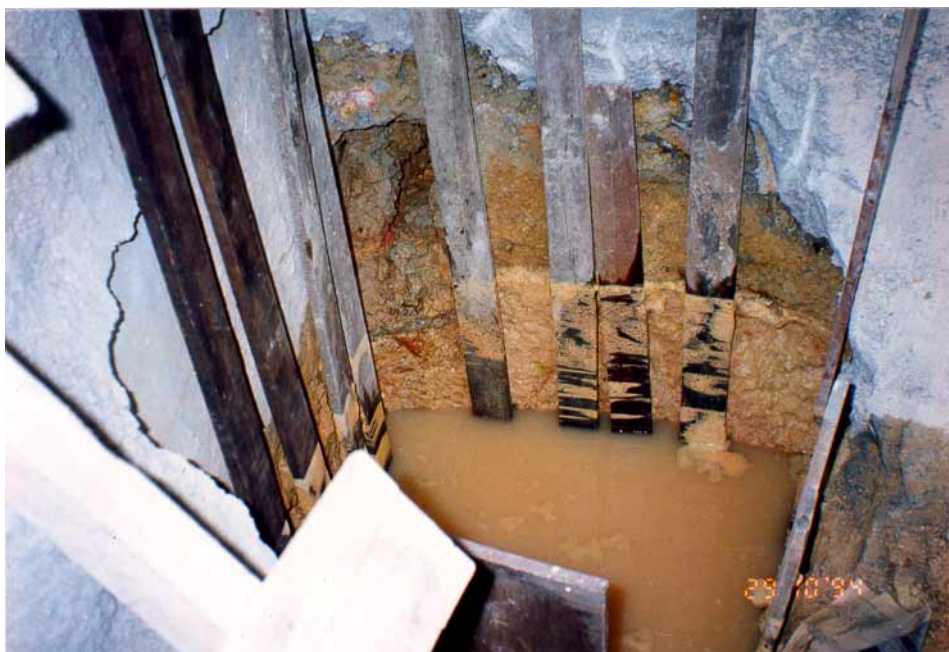
Plate M17 - Subsurface Seepage Flow into Trial Pit No. TP26 at the Crest of the Landslide Scar during the Water Test underneath Block D (Photograph taken on 29 October 1994)
