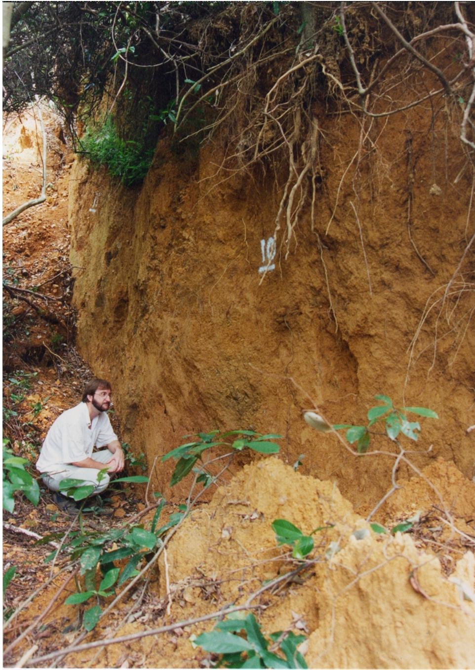
Plate 5 - Main Scarp, Vertical Displacement at this Point is 3.8 m (Taken on 26 September 1997)
