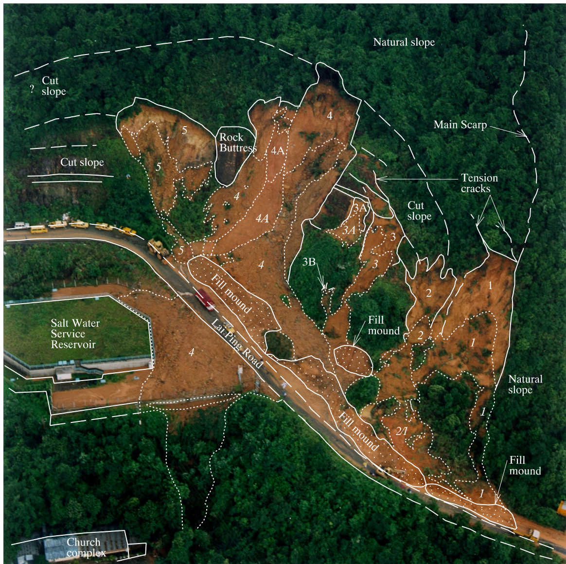
Plate 4 - Oblique Aerial View of Lai Ping Road Landslide (Annotated to Show the Landslide Scars 1-5 and Associated Debris and Part of the Main Scarp, Taken on 4 July 1997)
