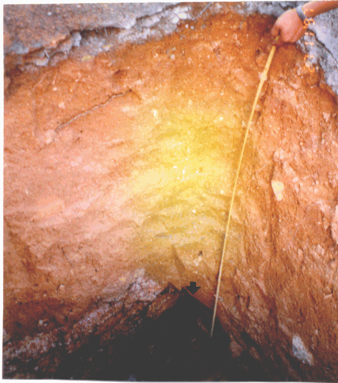
Plate 8 - Open Relict Joint about 80 mm Wide in Completely Decomposed Granite below Fill in Trial Pit No. TP1 (Photograph Taken on 27 November 1997)
