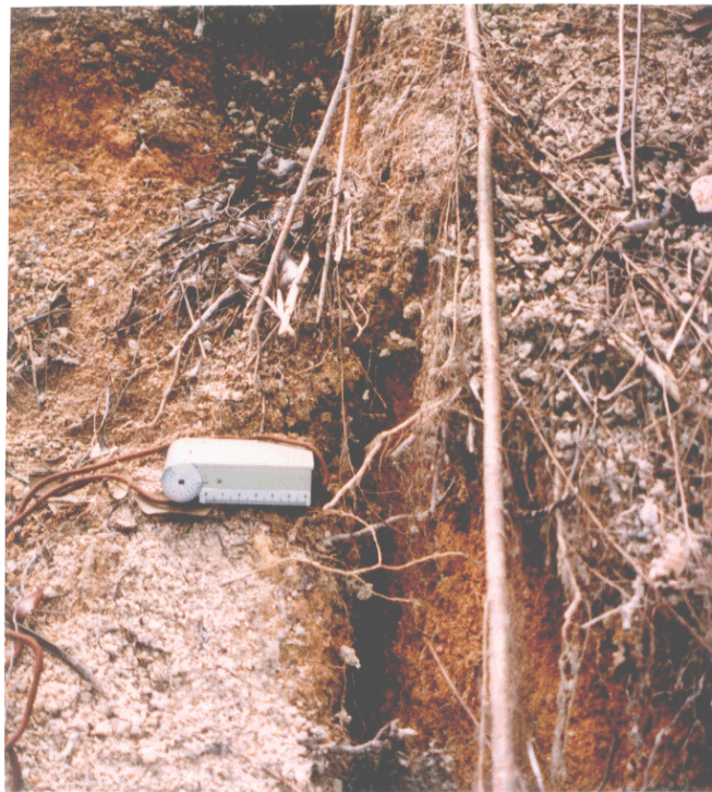
Plate 3 - View of Recent Displacement across Western Part of Tension Crack (Photograph Taken on 2 February 1998)
