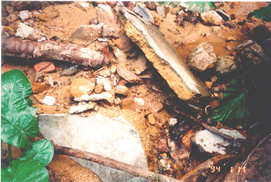
Plate 4 - Chunam Fragments Found at Toe of the Debris (Photograph Taken on 17 June 1997)
