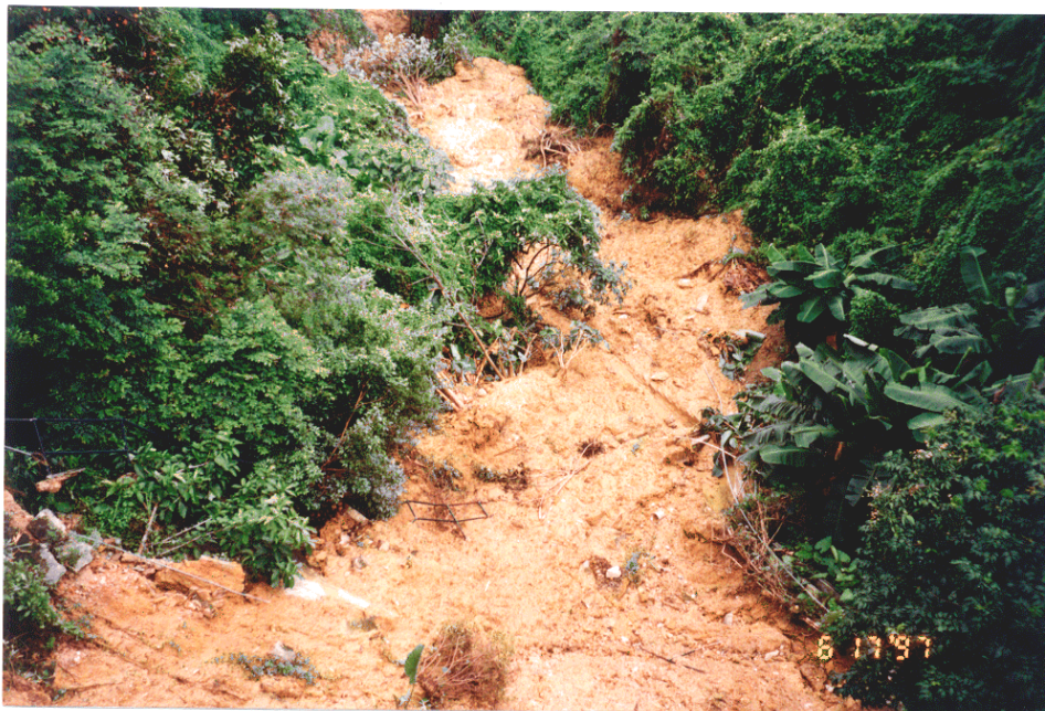
Plate 3 - View of the Track of the Landslide of 4 June 1997 (Photograph Taken on 17 June 1997) (Note Super-elevation of Debris on the Right Hand Side of the Elbow in the Debris Track)
