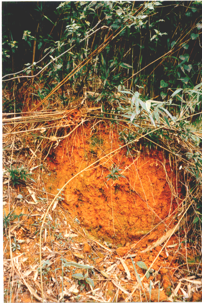
Plate 6 - Residual Soil Exposed by Erosion on the Slope Adjacent to the Landslide (Photograph Taken on 23 March 1998)
