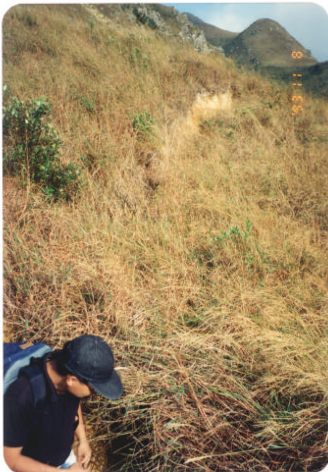
Plate 20 - Tension Crack at Small Displacement Landslide ( TP 231/19 )
