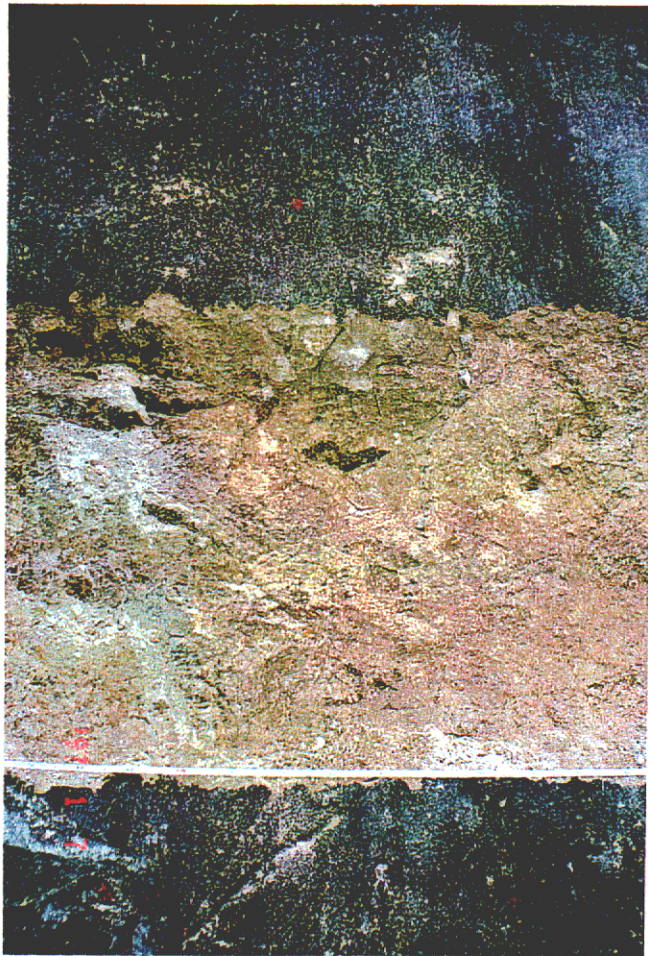
Plate 13 - Thin quartz vein within completely decomposed granite along chunam strip CSG1 at Site G. (Eg97/11/23)
