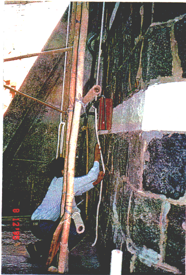
Plate D36 - SIR 2 System 500MHz monostatic antenna being held against masonry wall at Site B (TB01) during ground penetrating radar survey. Contractor Bachy Soletanche. (EG95/158/12)
