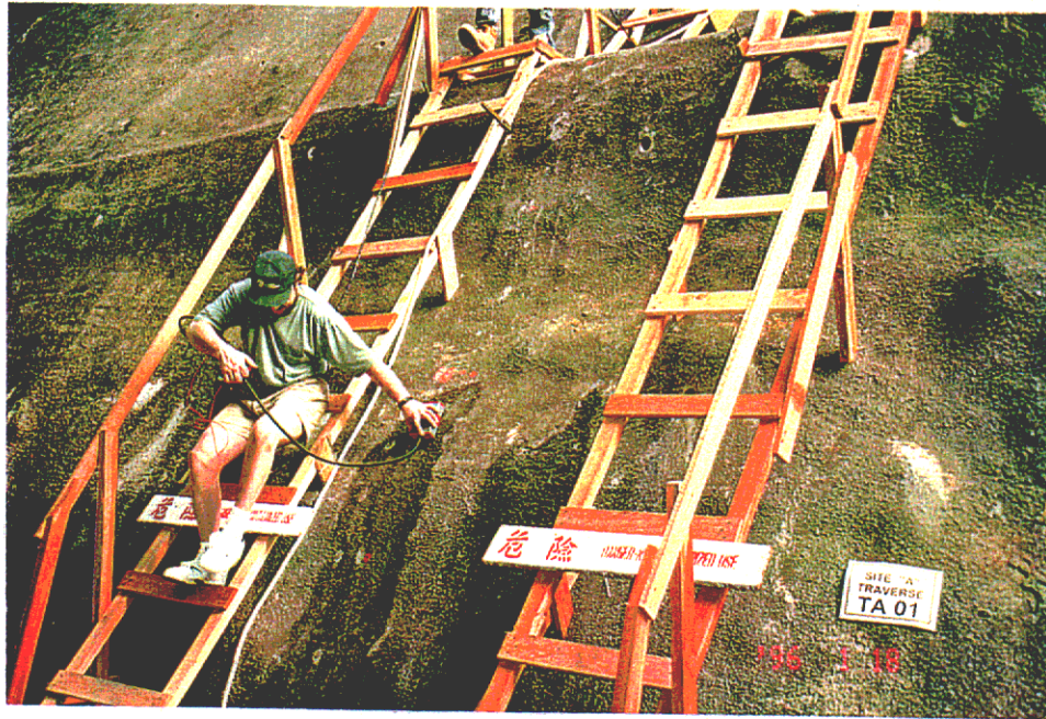
Plate D27 - 1GHz GSSI antenna being used to penetrate mesh reinforced shotcrete at Site A (TA01) - Contractor Golder Associates. (EG96/28/9)
