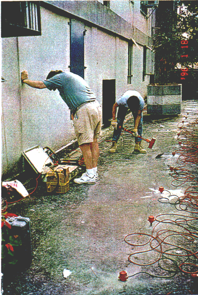
Plate D1 - 6 kg sledge hammer being used at Site A (TA04) as energy source for high resolution seismic reflection. Contractor Golder Associates. (EG96/28/21)
