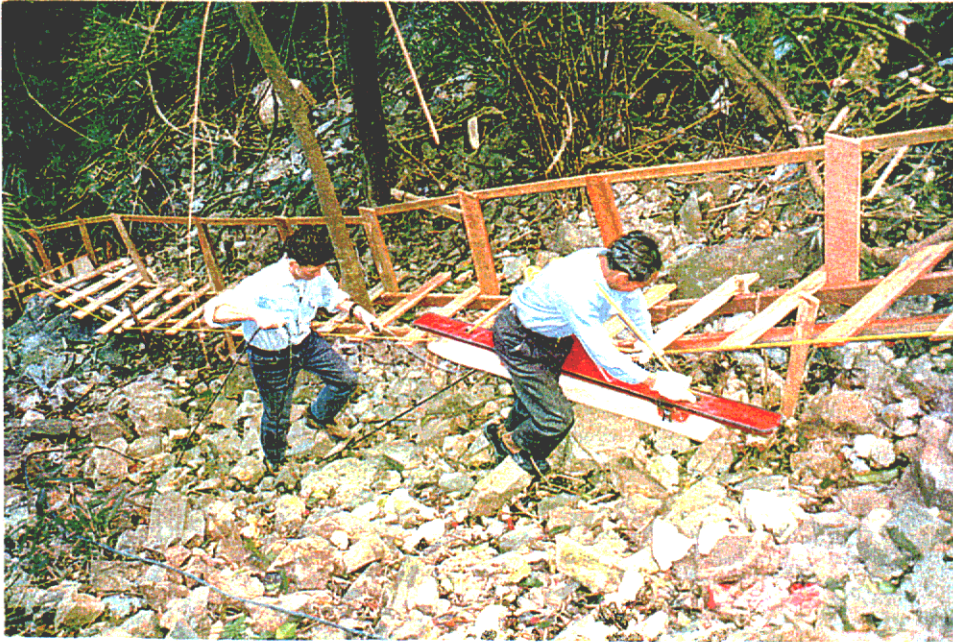
Plate D37 - Radarteam - Sweden A - Model subecho 40 - monostatic 35MHz non-contact antenna being used during GPR survey at Site D (TD02). This non-contact antenna has obvious advantages over the contact type of antenna in rough ground conditions. Contractor Fugro Geotechnical Services (HK) Ltd. (EG95/172/18)
