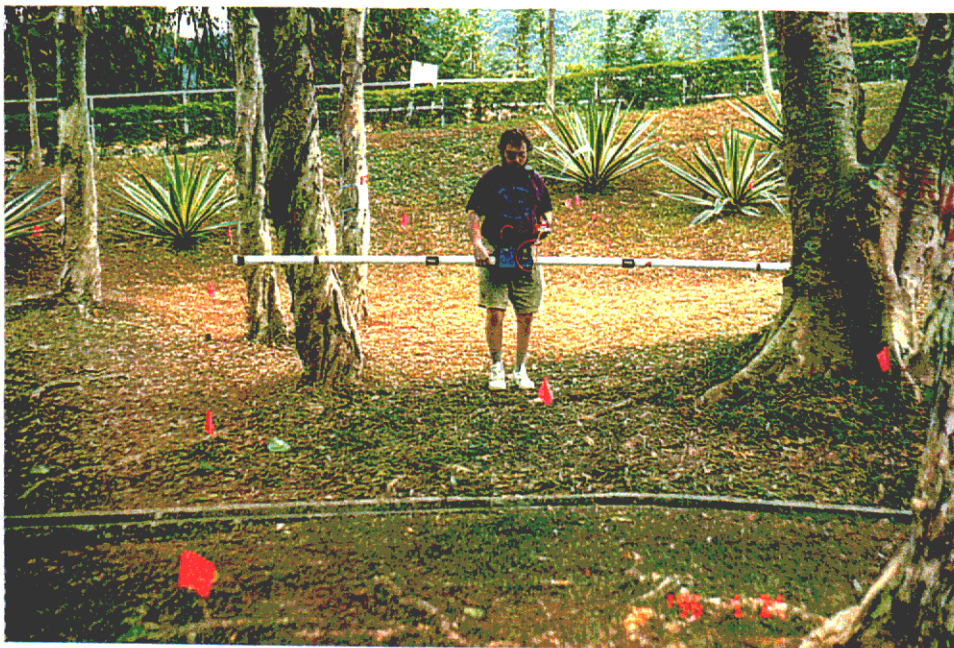
Plate D24 - Geonics EM-31 being used for FDEM survey of fill slope platform at Site D. Red flags define the 1m grid used to carry out the survey. Contractor Golder Associates. (EG96/39/4)
