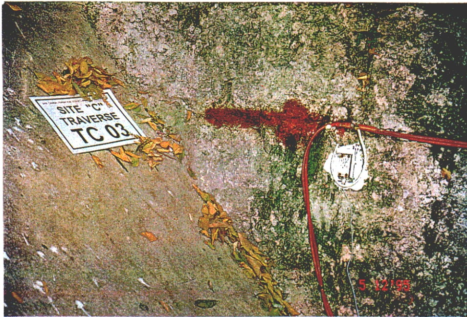
Plate D5 - Metravib CSH05 Piezoelectric accelerometer attached to masonry wall with plaster of Paris at Site C (TC03) during SASW survey. Contractor Bachy Soletanche. (EG95/143/14)
