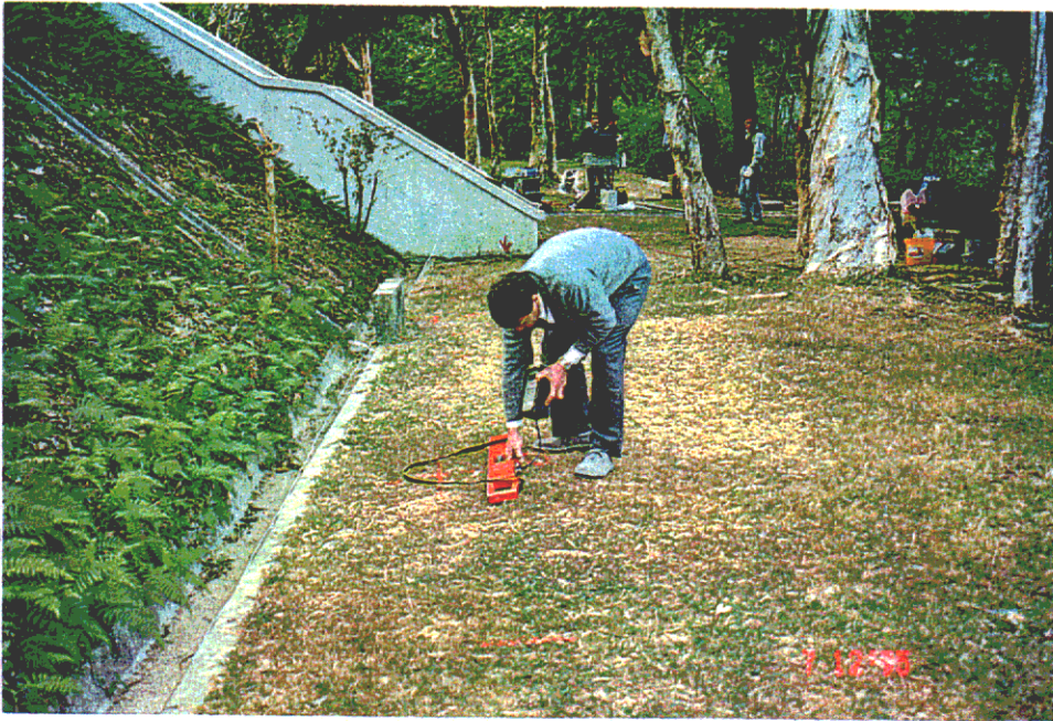
Plate D23 - Geonics EM38 conductivity meter being used at Site D (TD01). Contractor Bachy Soletanche. (EG95/155/19)
