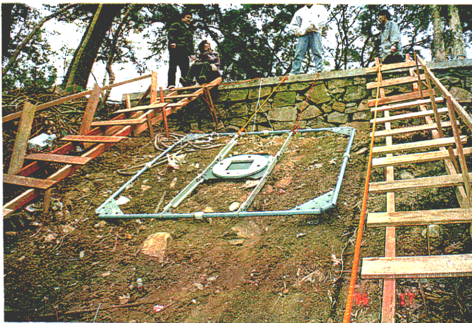
Plate D25 - Crone Geophysics & Exploration Ltd. digital pulse TDEM system being lowered down fill slope at Site D (TD02). Contractor Institute of Geophysical and Geochemical Exploration. (EG96/17/21)
