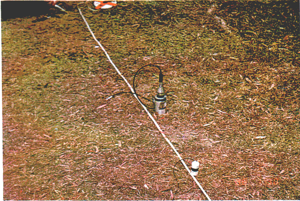
Plate D9 - Low frequency 1Hz geophone used to record long wavelength surface waves during SASW survey at Site D (TD01). Contractor Golder Associates. (EG96/45/6)
