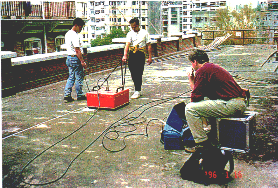
Plate D29 - GSSI 200MHz monostatic antenna being pulled along platform above the masonry wall at Site B (TB05) during GPR survey. Contractor Meinhardt Works. (EG96/12/8)
