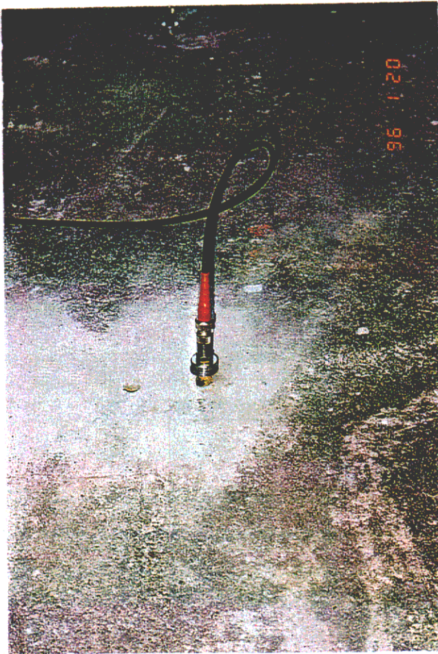
Plate D5 - Metravib CSH05 Piezoelectric accelerometer attached to masonry wall with plaster of Paris at Site C (TC03) during SASW survey. Contractor Bachy Soletanche. (EG95/143/14)
