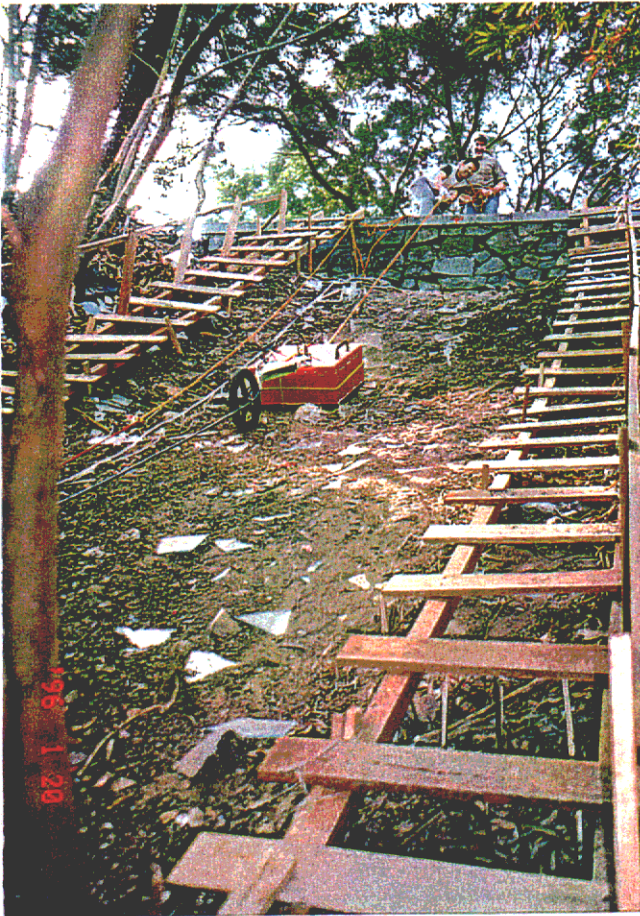
Plate D33 - GSSI 200MHz monostatic antenna being pulled up fill slope at Site D (TD02) during GPR survey. Note survey wheel attached which automatically encodes the radargram with a distance measurement. Contractor Meinhardt Works. (EG96/30/17)
