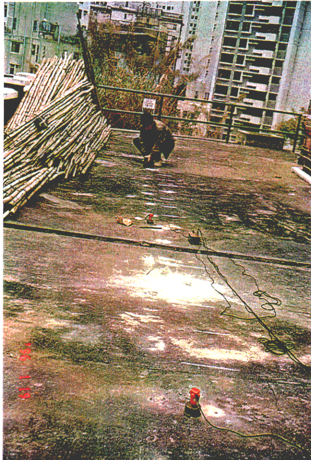
Plate D13 - Common mid-point receiver array being used for SASW survey at Site B (TB05). Sounding point is mid-way between the two geophones. Contractor Institute of Geophysical and Geochemical Exploration. (EG96/26/24)
