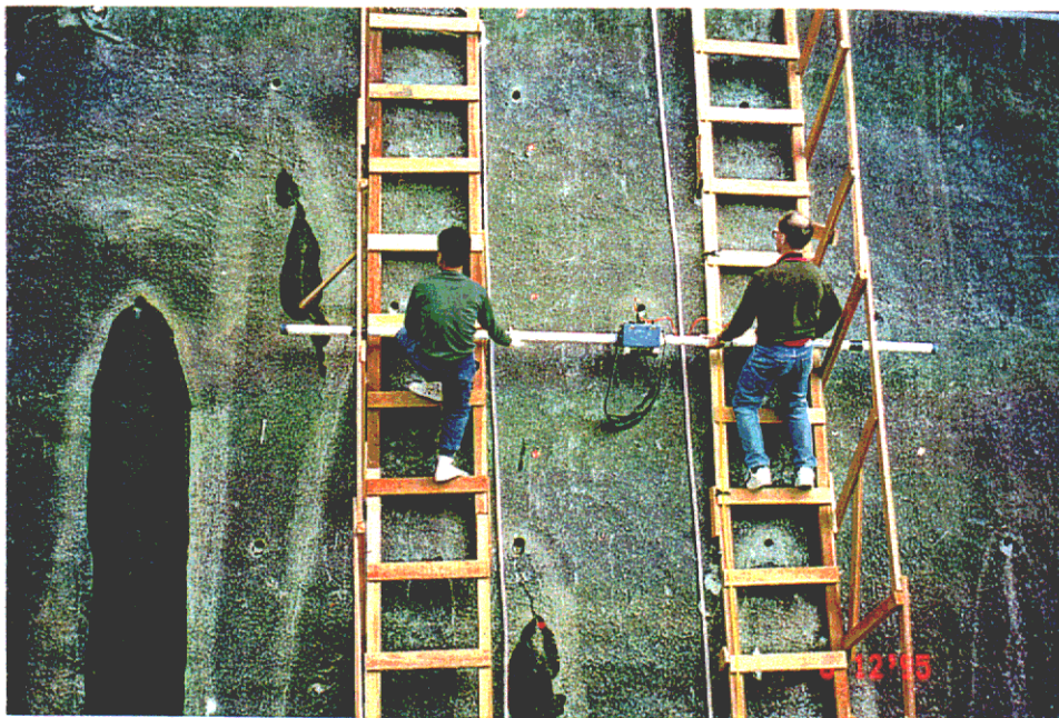
Plate D22 - Geonics EM31 conductivity meter being used at Site A (TA01). Two-man job to carry out the survey up the slope at the site. Contractor Fugro Geotechnical Services (HK) Ltd. (EG95/156/17)
