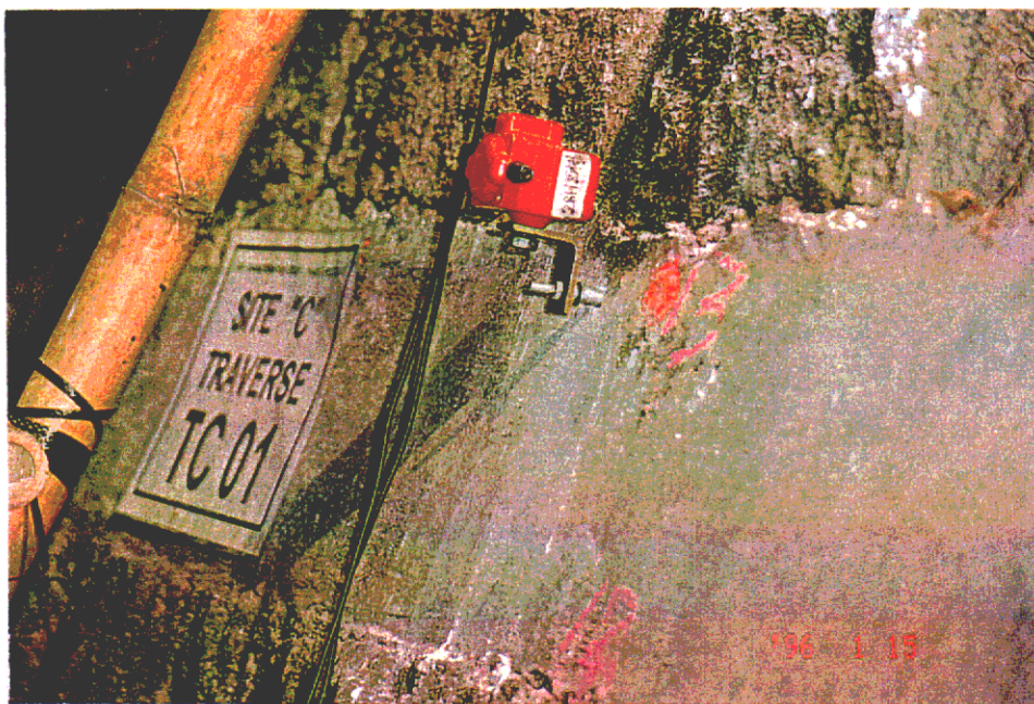
Plate D7 - SASW geophone inserted into pre-drilled hole along the masonry wall tie beam at Site C (TC01). Contractor Institute of Geophysical and Geochemical Exploration. (EG96/14/7)
