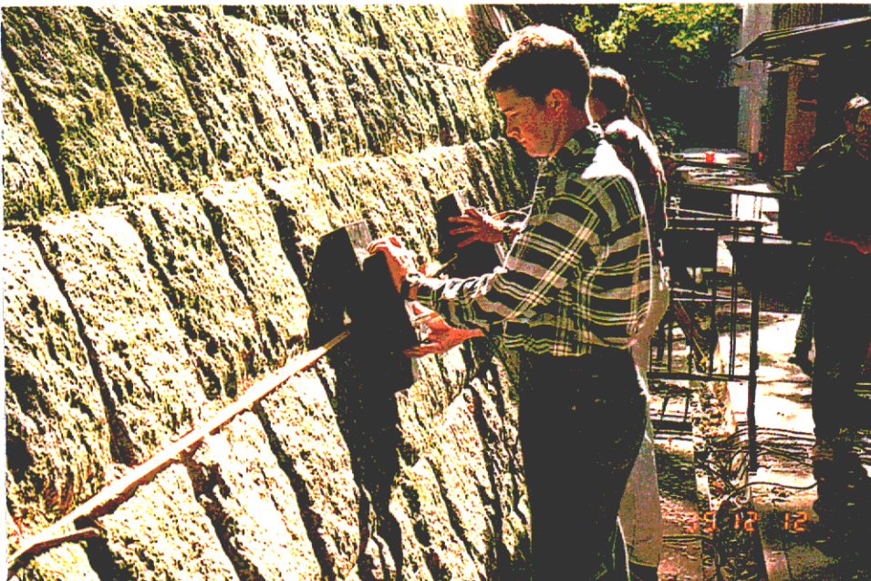
Plate D34 - Sensors & Software Inc. PulsEKKO 1000 System 225MHz antenna's being used in a Common Depth Point (CDP) GPR survey for masonry wall velocity determination at Site C (TC03). Contractor Fugro Geotechnical Services (HK) Ltd. (EG95/165/20)
