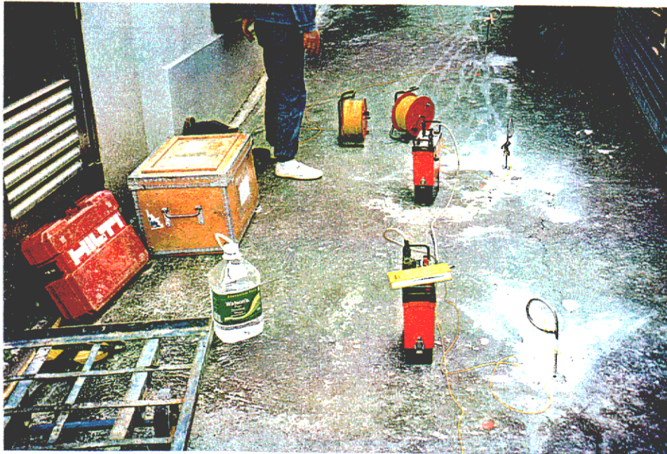
Plate D16 - Steel pin electrodes inserted through concrete slab to ensure contact with soil beneath at Site A (TA03) during resistivity imaging survey. Contractor Fugro Geotechnical Services (HK) Ltd. (EG95/159/8A)
