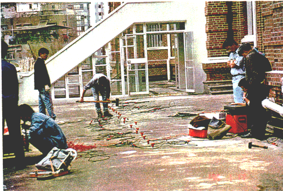
Plate D12 - SASW survey in progress with a multiple geophone array at Site B (TB04). Contractor Guandong South China EGT Co. (EG96/23/22)
