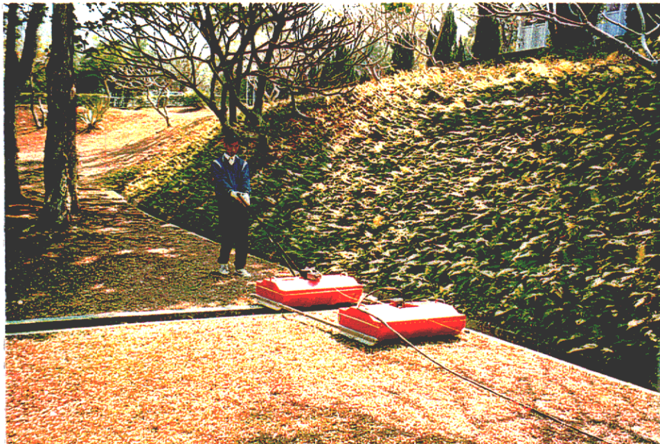
Plate D28 - GSSI 100MHz bistatic antenna being used in GPR survey at Site D (TD01). Contractor Guandong South China EGTD Co. (EG96/02/16)
