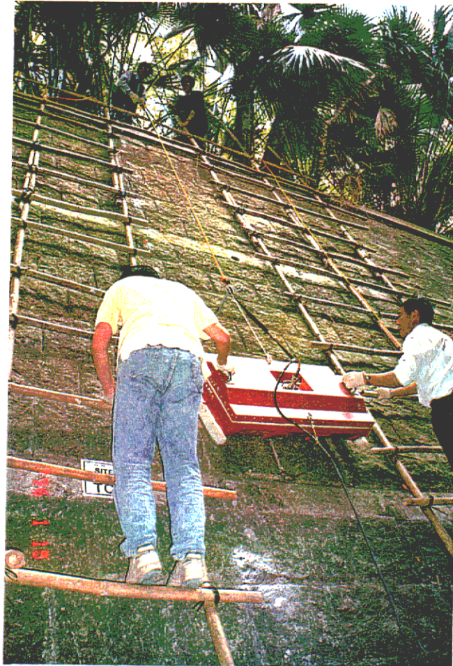
Plate D35 - GSSI 100MHz antenna being lowered down masonry wall at Site C (TC02). Note three men required to manhandle the large antenna to ensure proper contact with the wall. Contractor Institute of Geophysical and Geochemical Exploration. (EG96/11/8)
