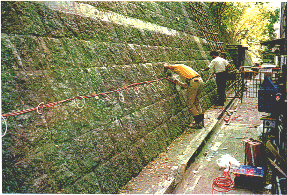
Plate D17 - Multi-takeout cable being attached to electrodes during resistivity imaging survey at Site C (TC03). This system allows each electrode to be identified so that surveys with different electrode spacing can be made automatically. Contractor Bachy Soletanche. (EG95/143/13)
