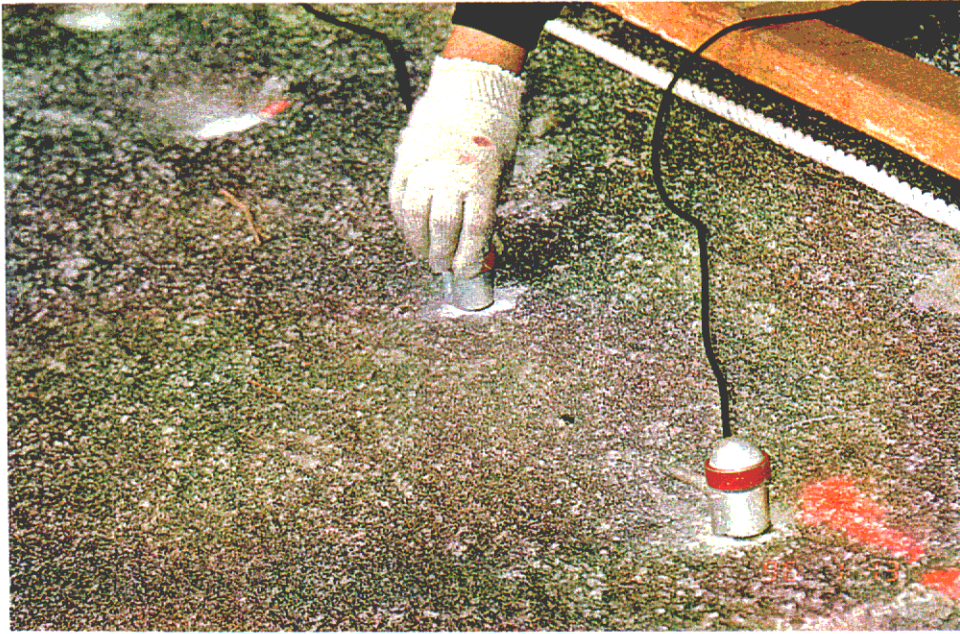
Plate D3 - 65Hz geophone being fixed to shotcrete slope surface during high resolution seismic reflection survey at Site A (TA01). Contractor Guandong South China EGTD Co. (EG96/08/23)
