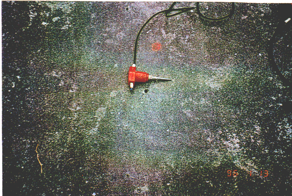
Plate D2 - Spiked geophone adjacent to pre-drilled hole prior to high resolution seismic reflection survey at Site A. Contractor Guandong South China EGTD Co. (EG96/07/20)
