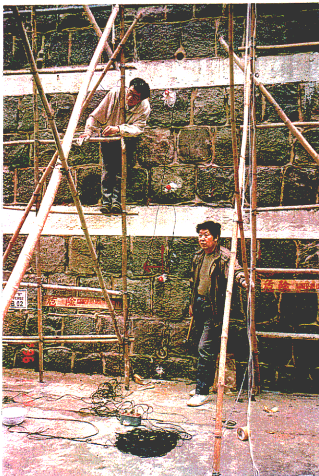
Plate D8 - Plaster of Paris being used to fix 10Hz geophones to masonry wall at Site B (TB02) during SASW survey. Contractor Institute of Geophysical and Geochemical Exploration. (EG96/27/20)
