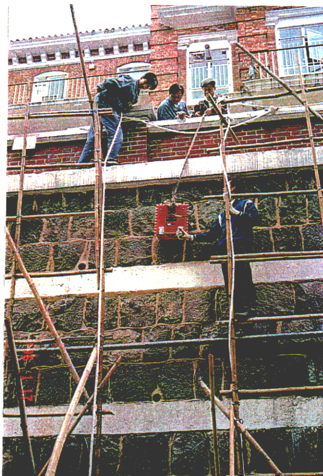
Plate D32 - GSSI 500MHz monostatic antenna being lowered down vertical masonry wall on a rope at Site B (TB02). Contractor Guangdong South China EGTD Co. (EG96/20/24)
