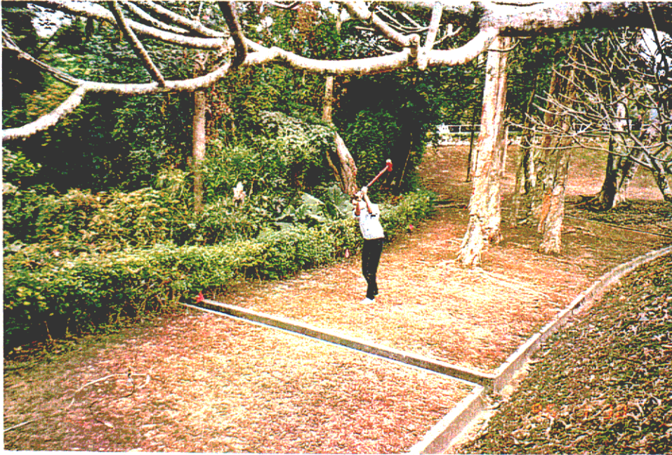
Plate D11 - 6kg sledge hammer being used at Site D (TD01) to produce low frequency surface waves during SASW survey. Contractor Golder Associates. (EG96/45/9)
