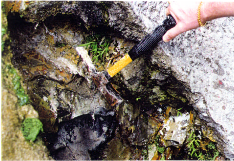
Plate 8 - Close-up (834255E 811530N) of Weathered Kaolinitic Clay Seam in Unregistered Slope 15NW-3B/S10, Lei Tung Estate as Shown in plate 3. (Taken 12/11/96)
