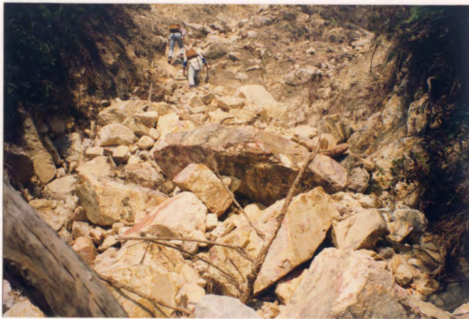
Plate B4.19 - Bouldery Debris Dammed by Big Boulders
