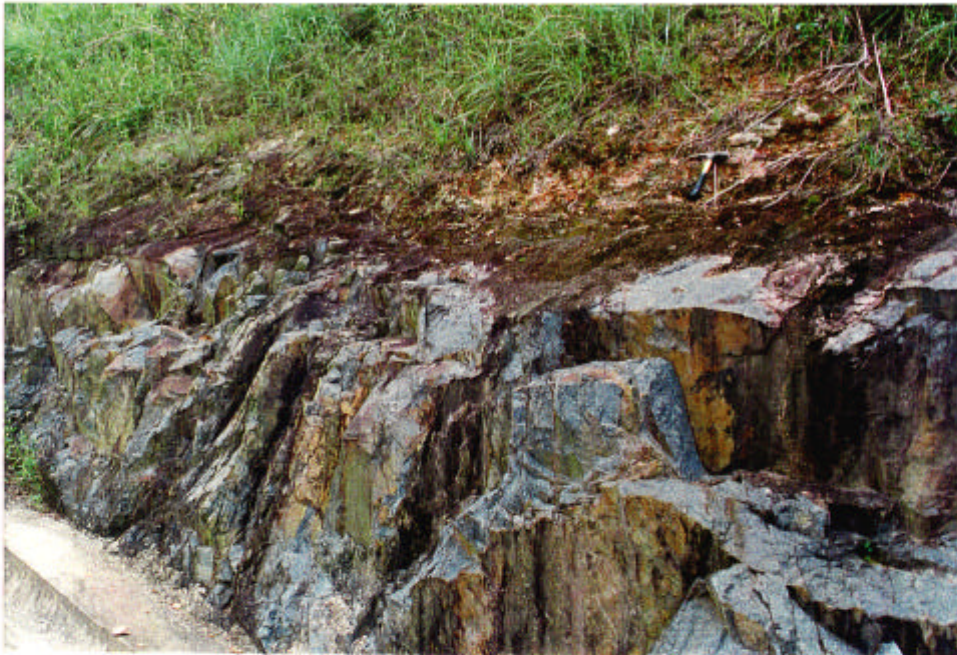
Plate 6 - General View of Outward-dipping, Planar PW0/30 and PW90/100 Rock Mass Weathering Zone Interface (843478 813884), Associated with Kaolinitic Clay Development, in Slope 11SE-D/C187, Northwest of Siu Sai Wan Estate (Taken 24/7/96)
