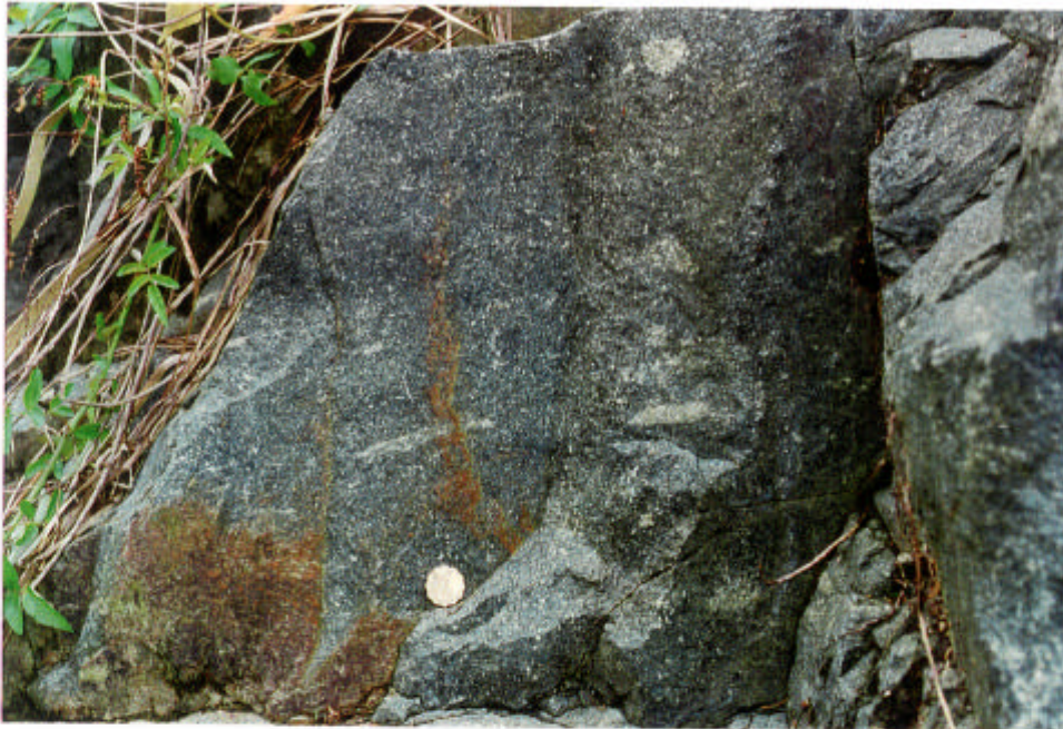
Plate 2 - Typical Volcanic Fabric with Aligned Lapilli and Fine Eutaxitic Foliation (844500 813614) in Slope 11SE-D/C181, Southeast of Siu Sai Wan Estate (Taken 26/6/96)
