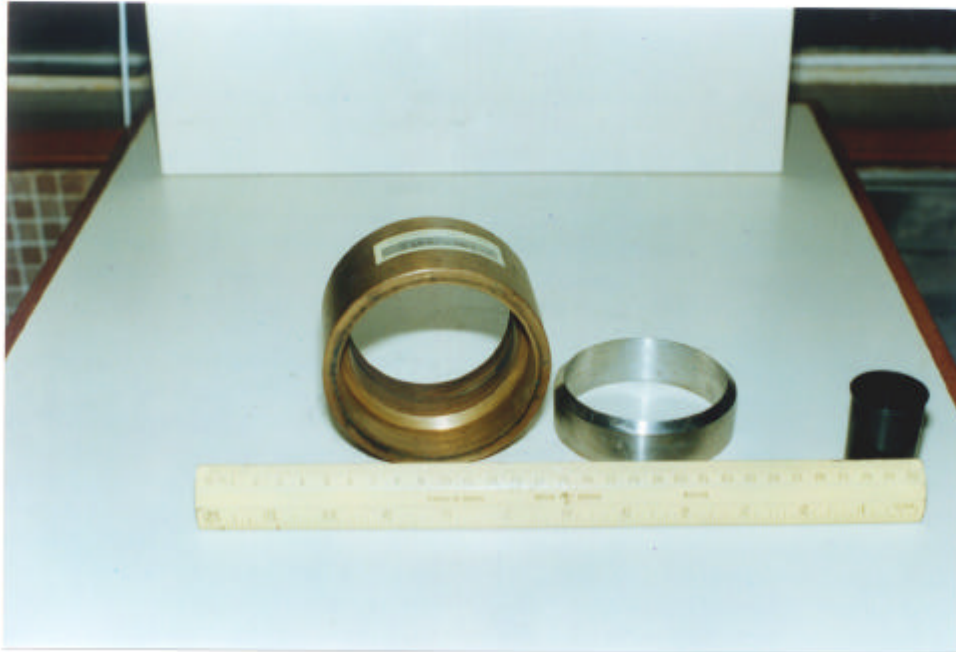
Plate 5 - Sample Cutting Ring for Rowe Cell A (Negative No. SP9202718)
