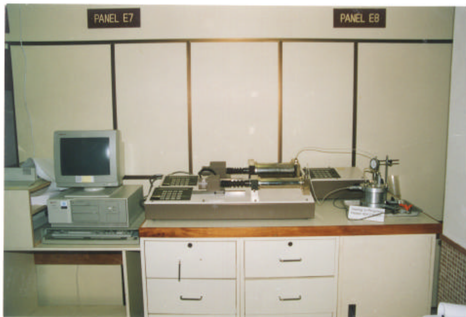
Plate 2 - Setup of the GDS Equipment for Continuous Loading Consolidation Test for Phase II Tests (Negative No. SP9411806)
