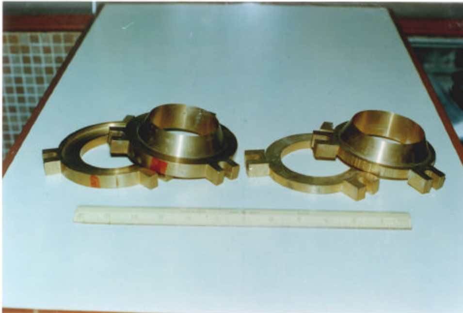
Plate 7 - Sample Cutting Shoe for Rowe Cell B (Negative No. SP9202700)
