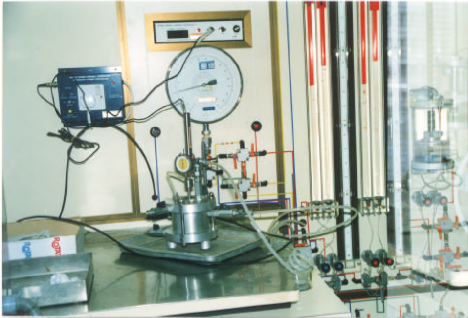
Plate 1 - Test Equipment for Rowe Cell Consolidation Test for Phase I Tests (Negative No. SP9226431)
