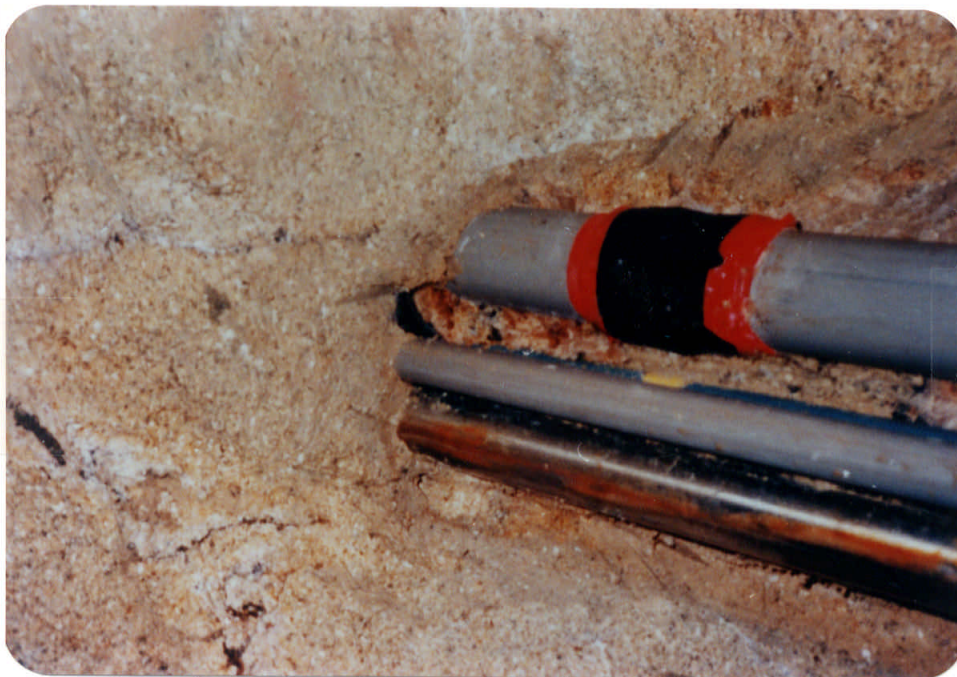
Plate 9 - Exhumed Grouted Drain D203B at Po Shan, Fully Sealed
