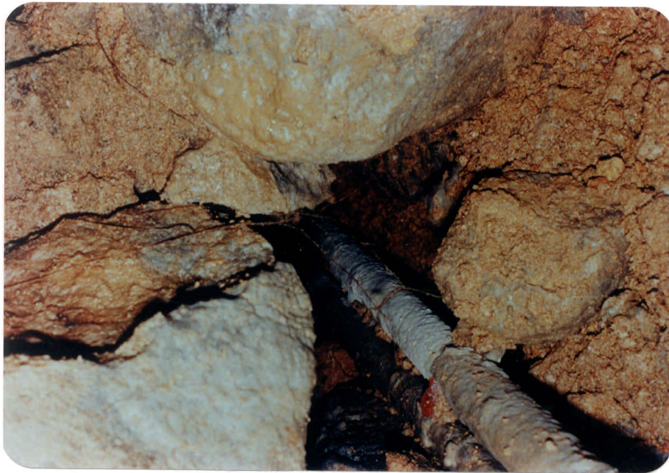
Plate 8 - Exhumed Grouted Drain D208 at Po Shan, with Surrounding Voids
