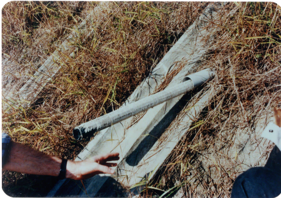
Plate 22 - Partly-exhumed Inner Liner from Drain at Tin Wan Hill Road
