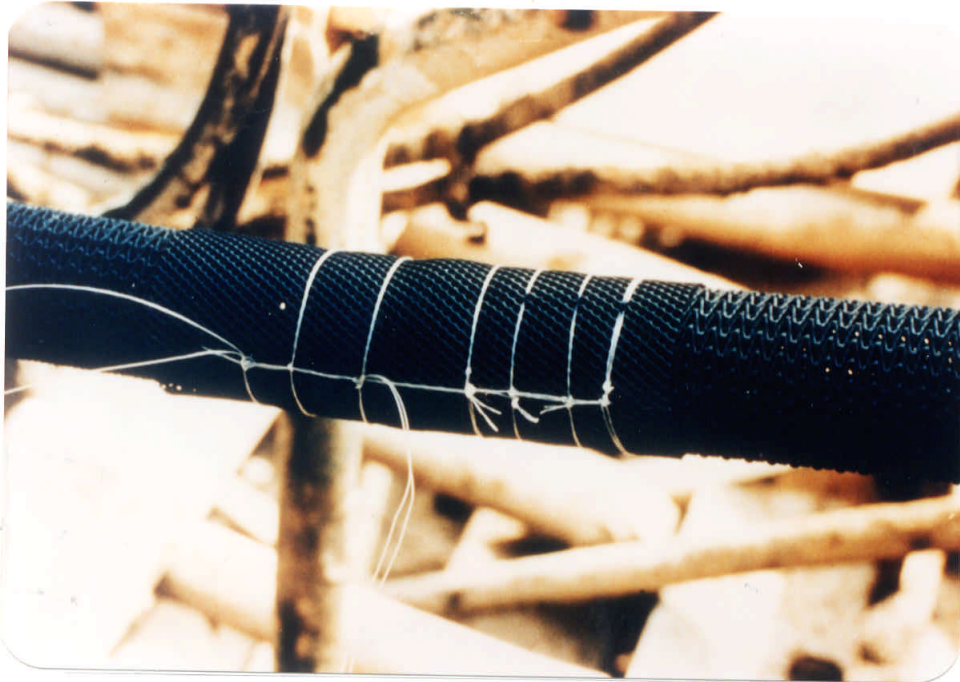
Plate 3 - Joint in GEO Type 3 Drain Liner Tied by Nylon Line
