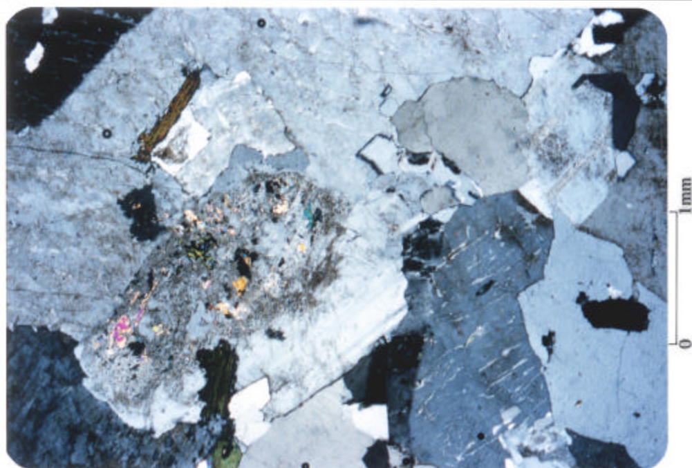
(a) Geological Survey Sample No. : 3614. Plagioclase (centre) showing sericitization; fresh alkali feldspar (streaky grey) and quartz (uniform grey or white); biotite (brown). (Cross-polarized light). Negative No. : SP 93/162/8A.
