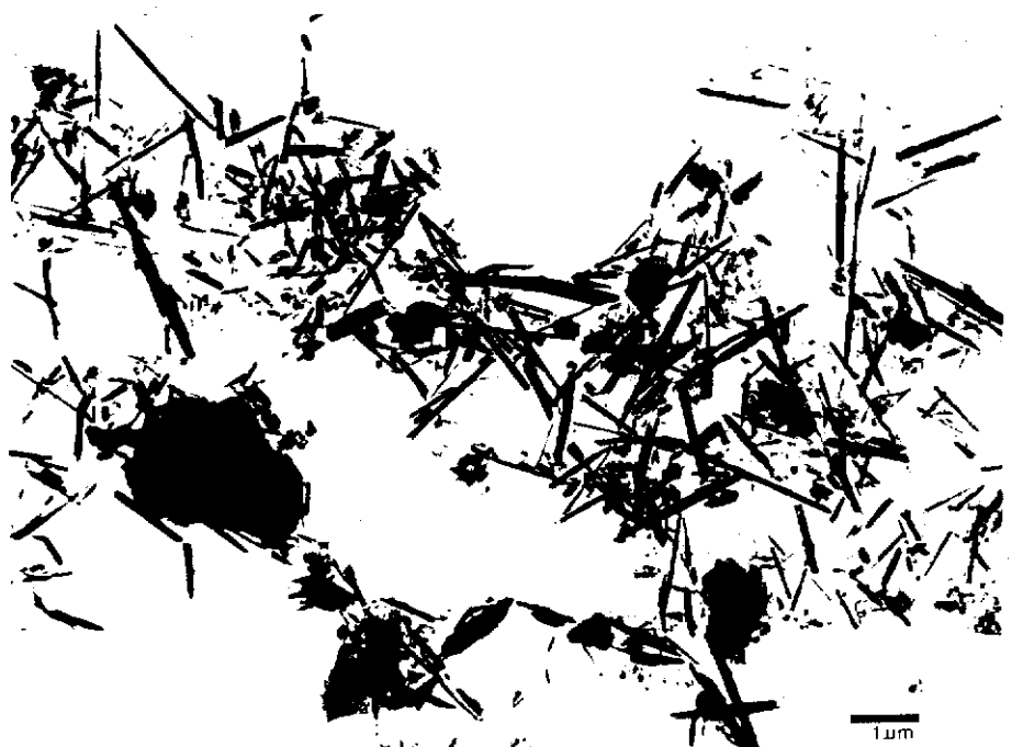
(b) Higher proportion of platy clay minerals in near surface completely decomposed (disintegrated) granite sample 404.07 from Shouson Hill. Negative No. : SP 93/167/5.
