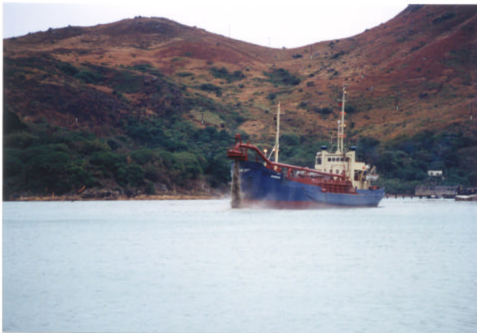
Plate 3.2 - Hydraulic Filling by Spigotting
