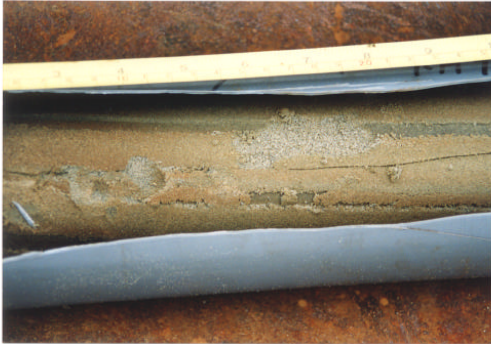
Plate 3.1 - Undisturbed Sample Obtained by Mazier Sampler (CS1)
