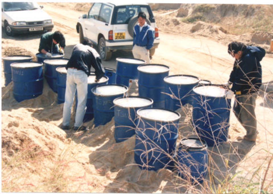
Plate 4.2 - Steel Barrels Holding Marine Sand Fill to be Shipped out to Italy for Stress Chamber Testing
