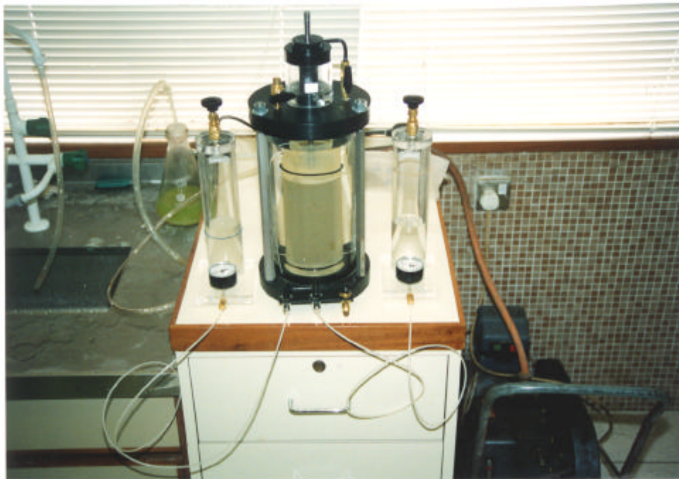
Plate 5.2 - Dual Evacuation Chambers Method for Sample Saturation
