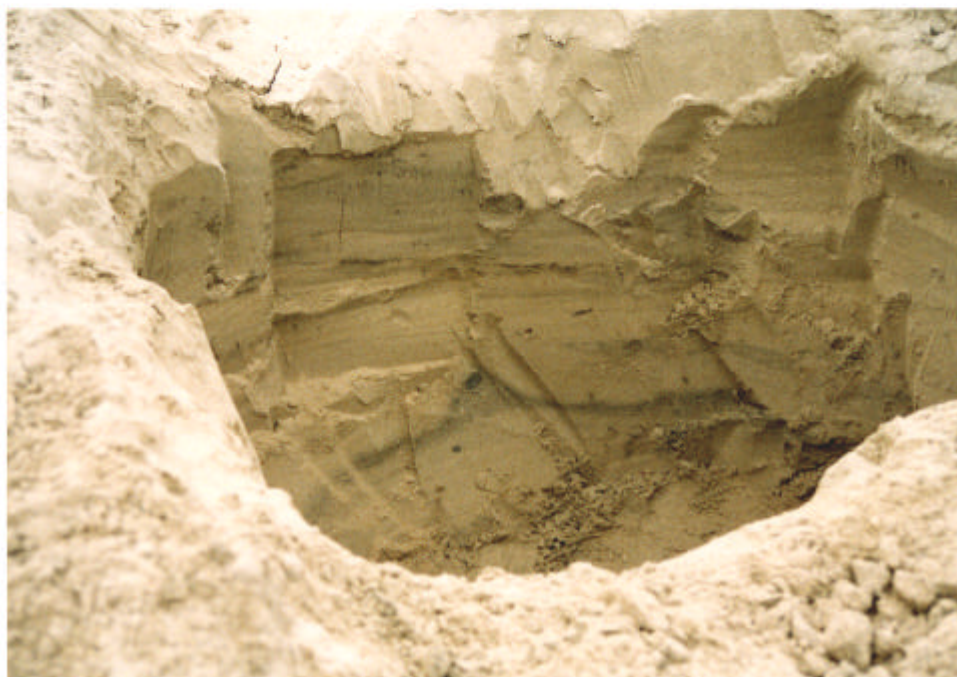
Plate 4.4 - Segregation Marks of Fine-to-coarse Sands at the Tseung Kwan O Site
