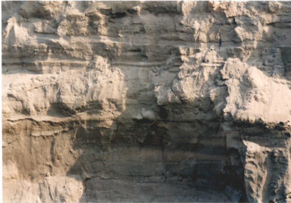
Plate 4.3 - Segregation Marks of Fine-to-coarse Sands at the West Kowloon Reclamation Site
