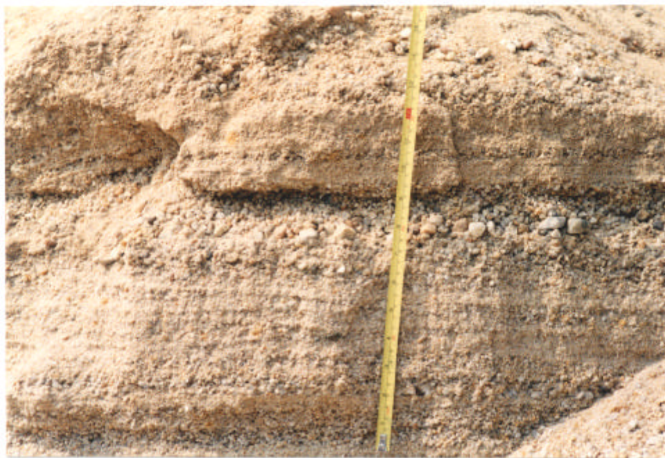
Plate 4.5 - Segregation Marks of Fine-to-coarse Sands at the Tin Shui Wai Site
