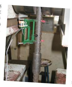
新的鋼筋連接器試驗 New test on reinforcement connectors
