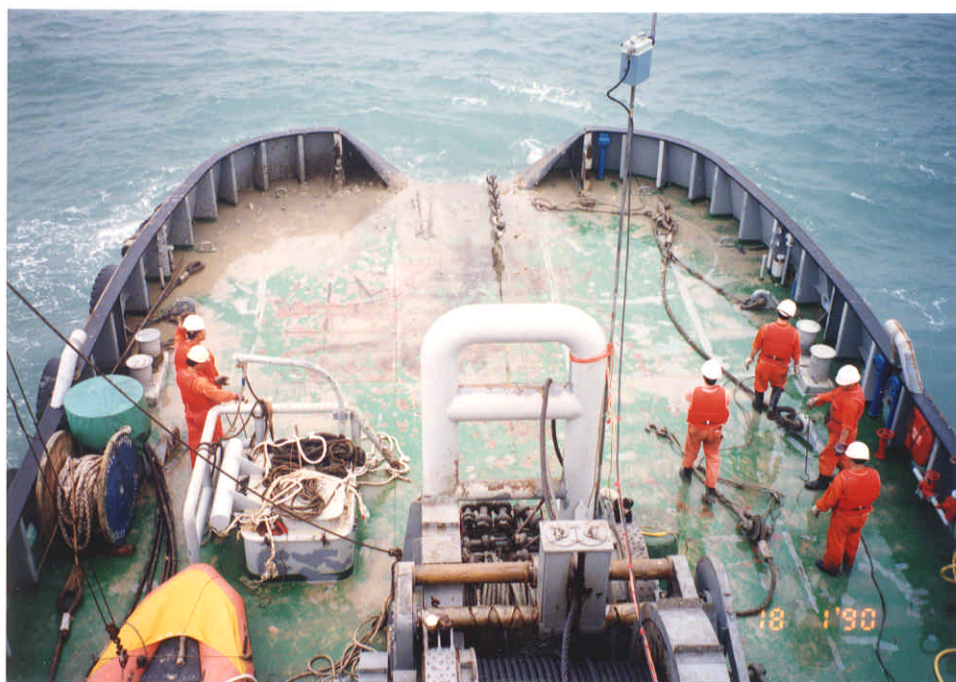
Plate 4 - Anchor-handling Tug the 'Tai-O' Deploying the Anchor System during the Trials at Urmston Road Borrow Area
