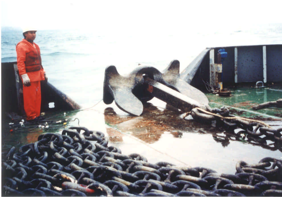
Plate 5 - The 3.4 Tonne OSS Type Test Anchor
