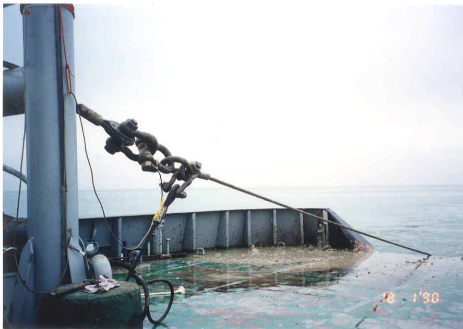
Plate 6 - Calibrated Load Shackle Fitted to Anchor Wire System
