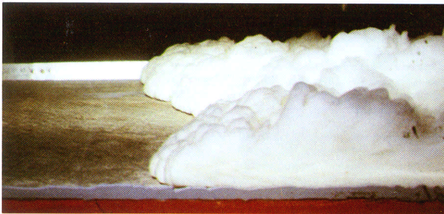
Figure 8. Model research into the transport of silt in water showed clearly that a density current can act as a transport mechanism; transportation of silt in this manner can be observed on this photograph. This research was carried out by the Delft Hydraulics Laboratory
