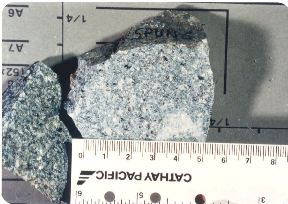
Plate 8 - Close-up of SPUN 6 Bulk Sample Fine Ash/Eutaxite Tuff Lithology (HK 8506)
