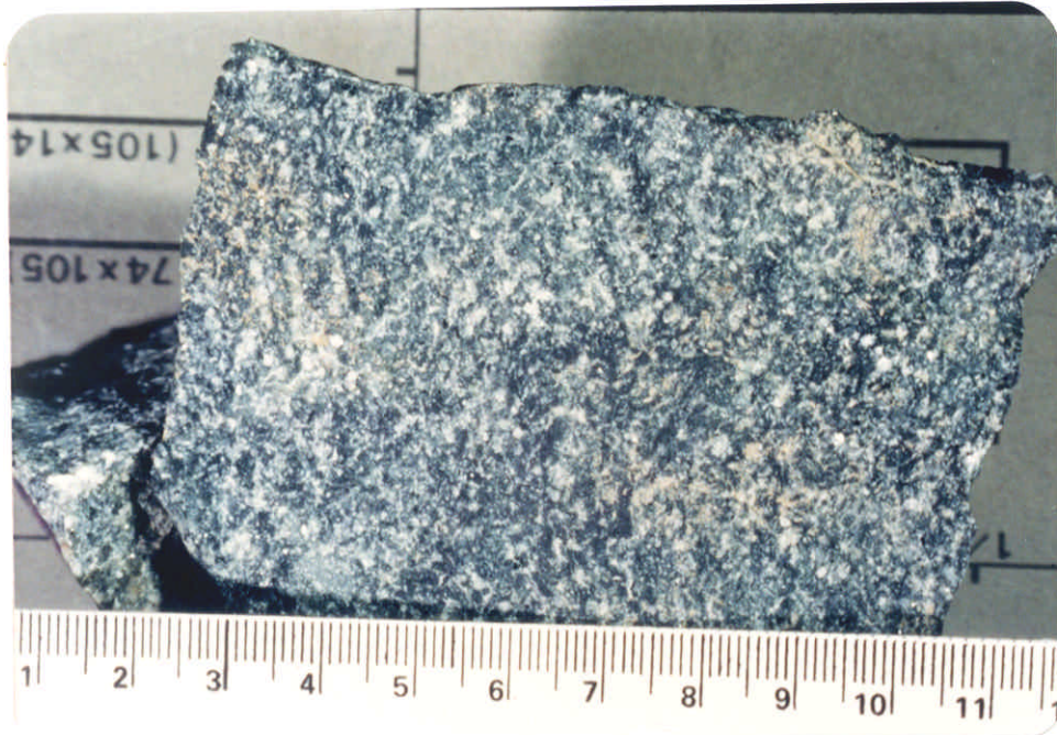
Plate 6 - Close-up of SPUN 4 Bulk Sample Fine Ash Tuff Lithology (HK 8504)
