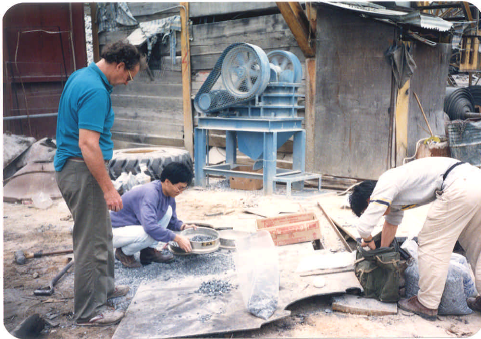
Plate 5 - Production of Aggregate for Testing by Field Crushing and Hand Sieving
