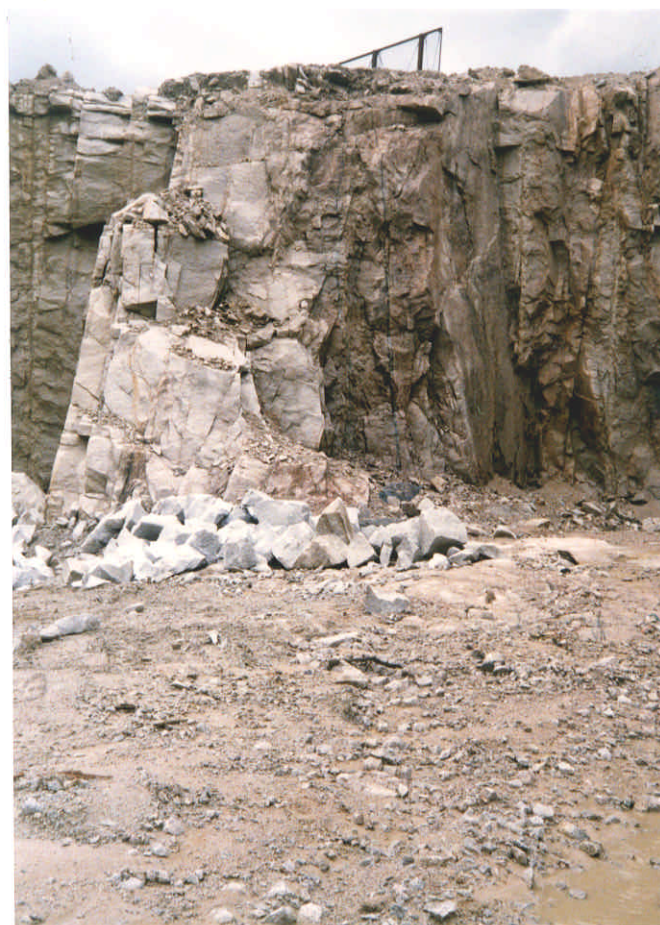
Plate 2 - Sampling Locality Showing the General Joints Distribution
