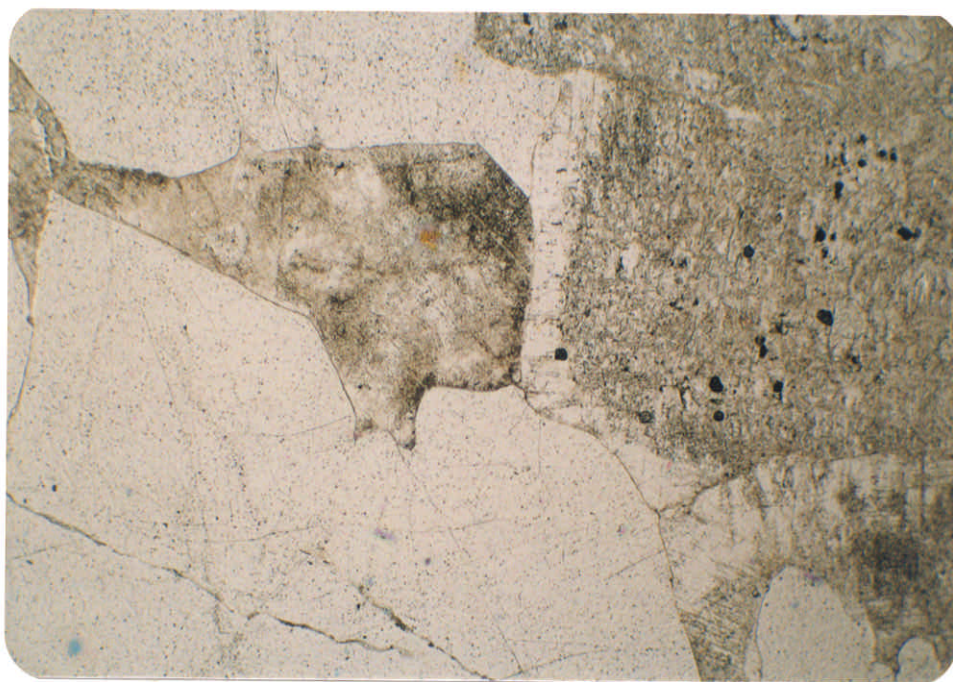
Plate 7b - Photomicrograph of Fine- to Medium-Grained Granite Showing Stained Grain Boundaries and Stained/Clean Transgranular Microcracks Plane Polarized Light - Enlarged Approximately 100 Times)
