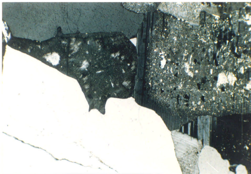
Plate 7a - Photomicrograph of Fine- to Medium Grained Granite Showing Transgranular Microcracks Through Quartz and Feldspar Grains. Plagioclase Feldspar (Right) is Partially Altered. K-feldspar (Centre) is Fresh (Enlarged Approximately 100 Times)
