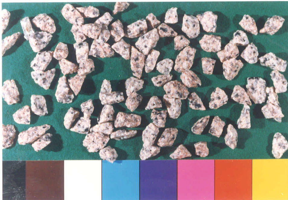
Plate 4 - Crushed Rock Aggregate from Fine- to Medium-Grained Granite
