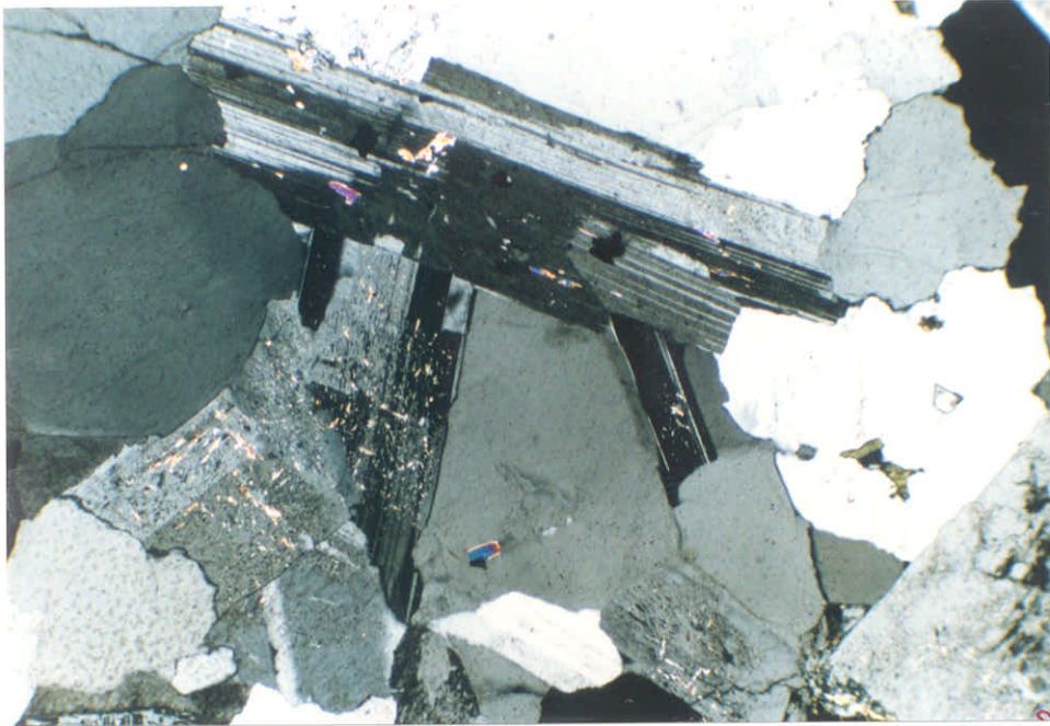
Plate 5a - Photomicrograph of fine-to medium-grained granite showing equigranular texture, alteration in plagioclase and grain boundary relationship (enlarged 100 times)
