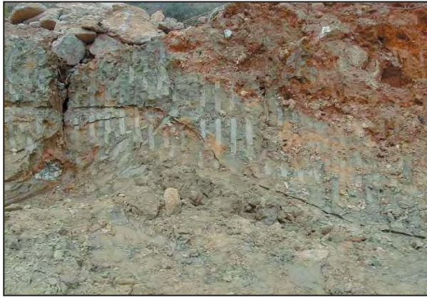
Figure 6.3.11 – Undulating Type 2 shear surface within completely decomposed andesite (photograph by N.P. Koor)
