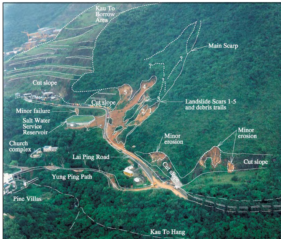
Figure 6.4.38 – 1997 shallow failures at Lai Ping Road and location of main scarp of older landslide (Sun & Campbell, 1999)
