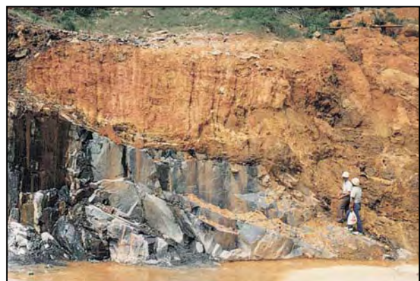
Figure 4.4.5 – Sharply-defined rockhead with little corestone development in volcanic rock. A possible kaolin-rich zone lies directly above rockhead (Fyfe et al., 2000)
