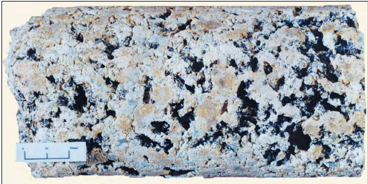
Figure 4.3.4 – Kaolinised granite core from the 1997 Ville de Cascade landslide site at Fo Tan (HAPL, 1998a)
