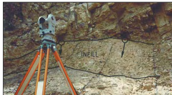
700 mm thick infill along rupture surface overlain by highly to moderately decomposed tuff with soil pipes that flowed with water for several days after the failure (indicated by arrows)
