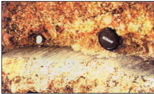
Figure 6.4.7 – Laterally persistent discontinuity infilled with slickensided kaolin and manganese oxide deposits at the toe of the Shek Kip Mei landslide (FMSW, 2000)
