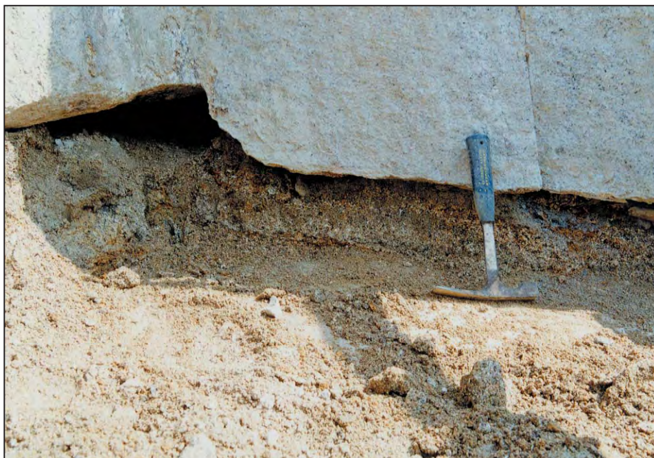
Figure 4.4.14 – Bedded granular material infilling sheeting joint
