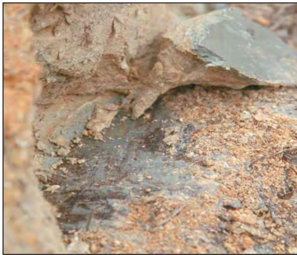
Figure 6.3.12 – Close-up of a Type 2 shear surface with polished and slickensided surfaces and grey clay infill (photograph by N.P. Koor)
