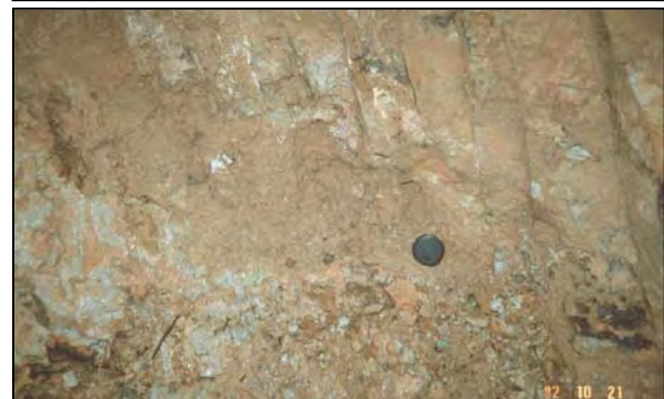
Completely to highly decomposed tuff fragments in a silt/clay matrix overlain by very closely jointed moderately decomposed tuff
