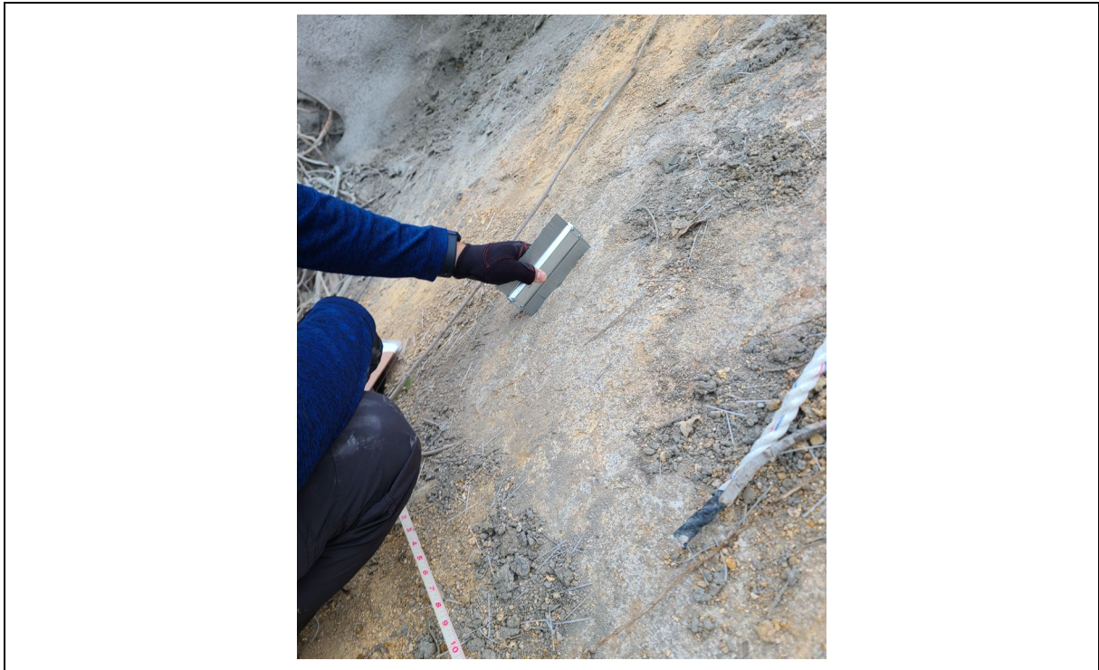
Figure 8.5 Field Measurements of Surface Roughness Using a Profilometer
