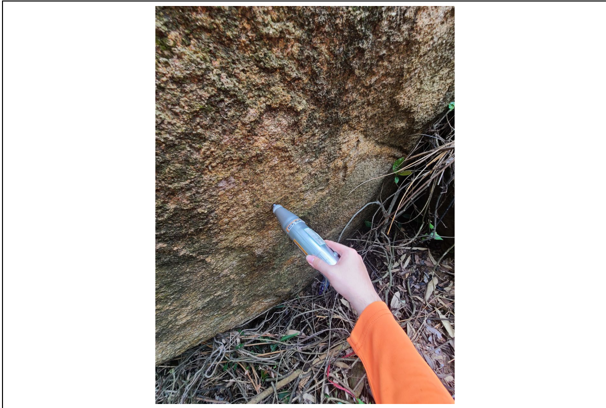
Figure 8.7 Schmidt Hammer Testing on a Tor
