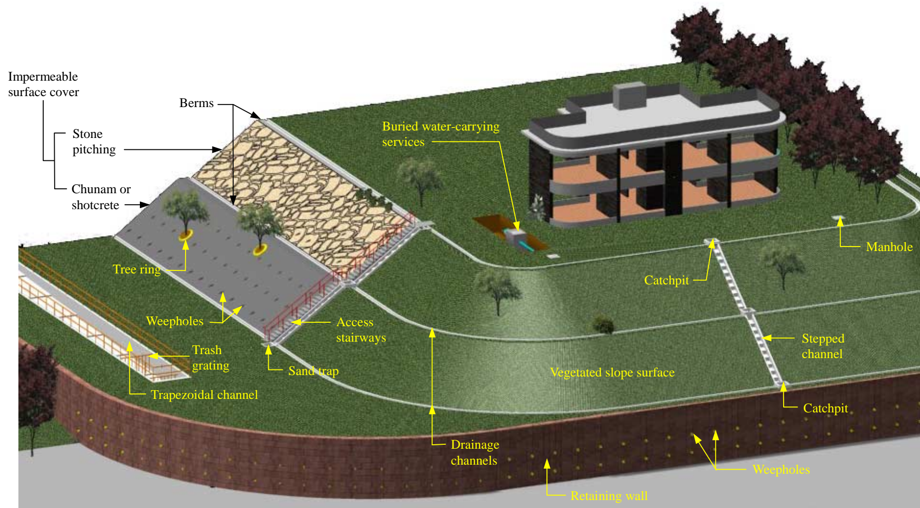
Figure 3.1 Typical Man-made Items on Slopes and Retaining Walls that Require Maintenance
