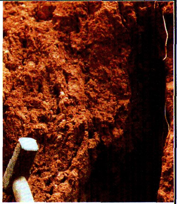
B: Microfractures Caused by Recent Slope Failure in a Volcanic Residual Soil at Pun Shan Tsuen, near Tsuen Wan, New Territories
