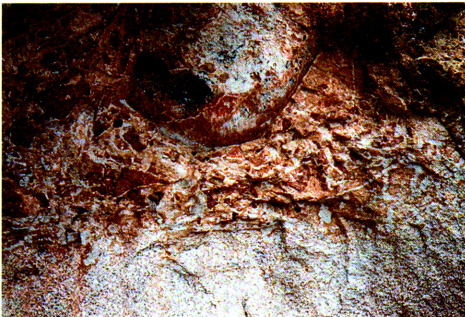
B: Boundary in a Trial Pit at Ngau Chi Wan, East Kowloon (Variably coloured (mottled), volcanic colluvium containing large decomposed boulders of ash tuff overlying uniform, light pinkish grey, completely decomposed medium-grained granite )
