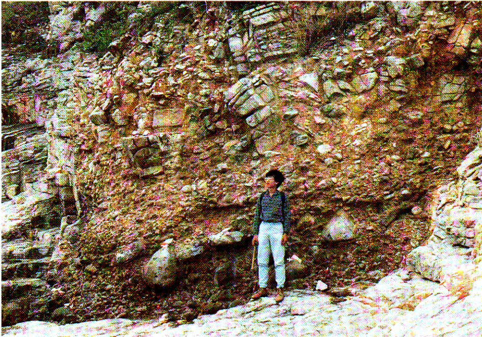
E: Field Exposure of Colluvium, Infilling a Small Valley on Ap Lei Chau, Hong Kong Island
