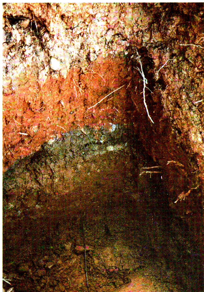
G: Exposure of Layered Fill in a Trial Pit at Peak Road, near Magazine Gap, Hong Kong Island
