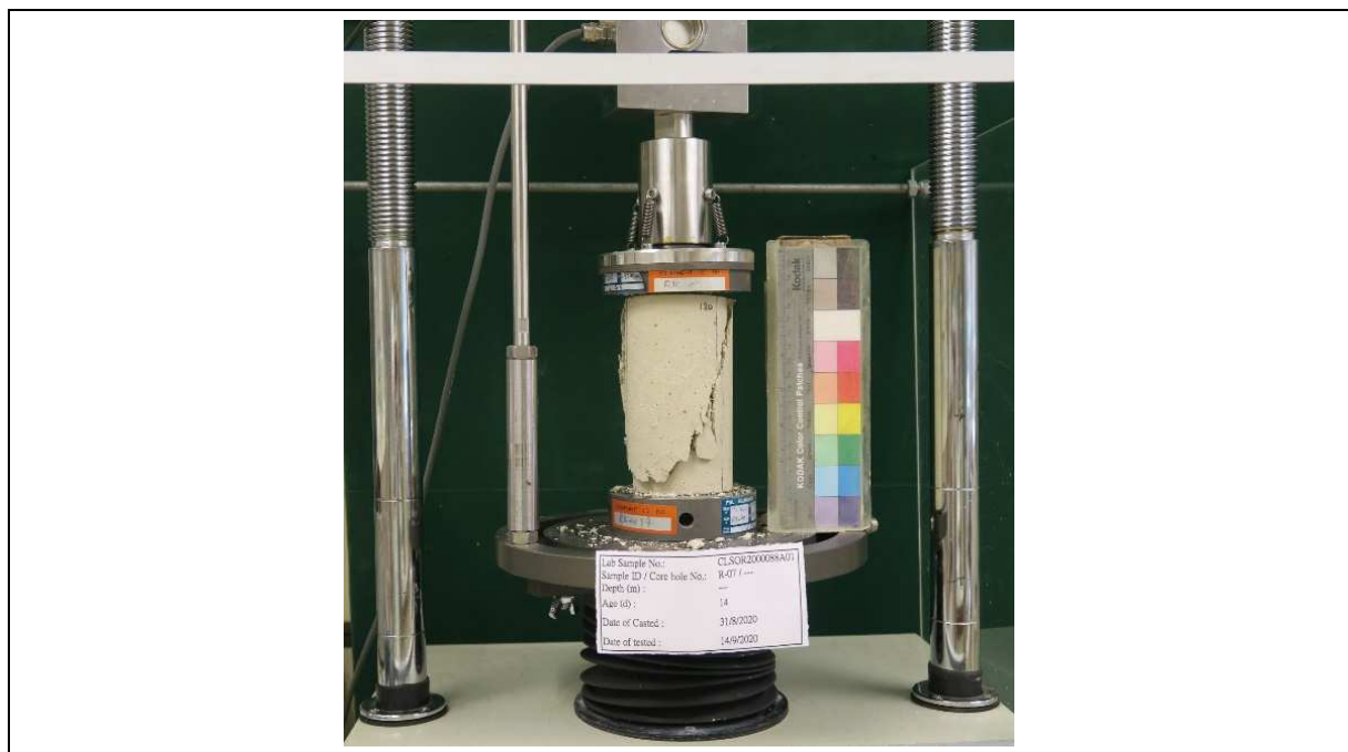
Figure 3.1 Unconfined Compressive Strength Tests of Cylindrical Specimen of Self-compacting Backfill Material
