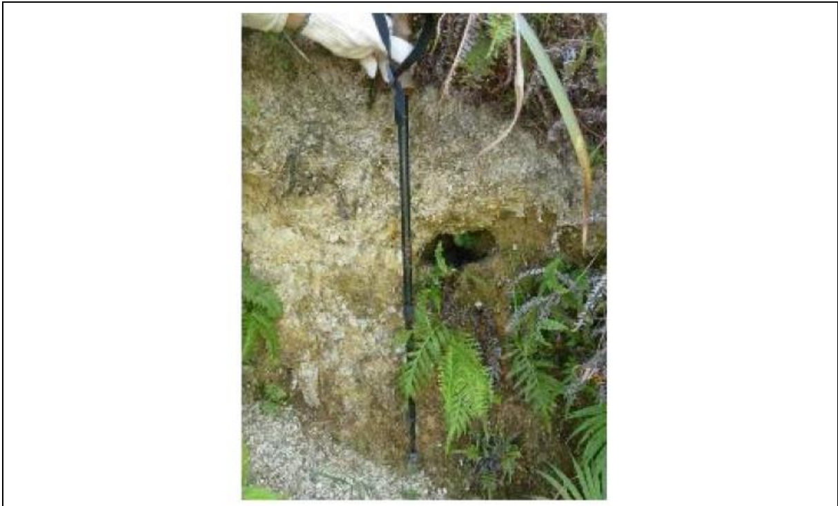
Plate D4.3 Soil Pipe (0.2 m in dia. And 0.5 m deep) Observed on the Scarp of Landslide Recent ENTLI No. 13NWB2013E (Landslide ID No. 51 in Catchment KSR56)
