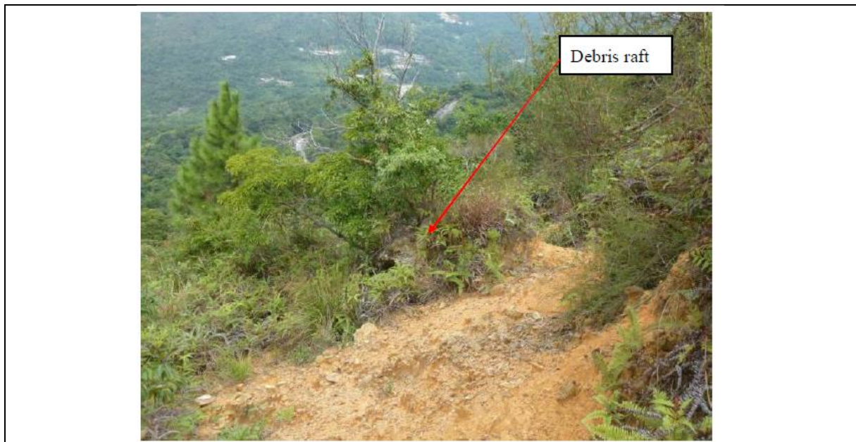
Plate D4.8 Displaced Intact Debris Raft on Recent Landslide ID No. 135 in Catchment KSR56A
