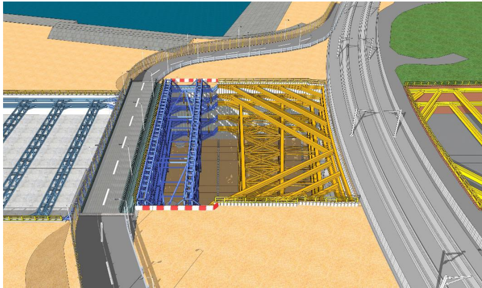
Figure 4.1 Use of BIM for the Cut-and-cover Tunnels in the Hong Kong International Airport
