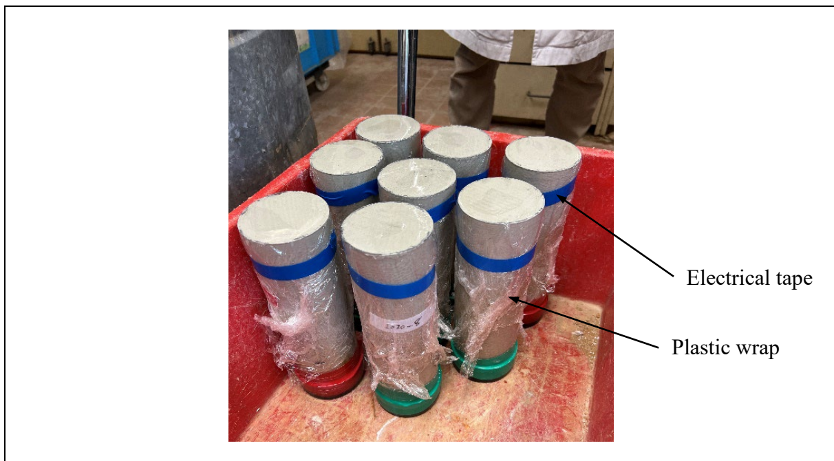
Figure 4.9 Specimens Covered by Sealant for Curing
