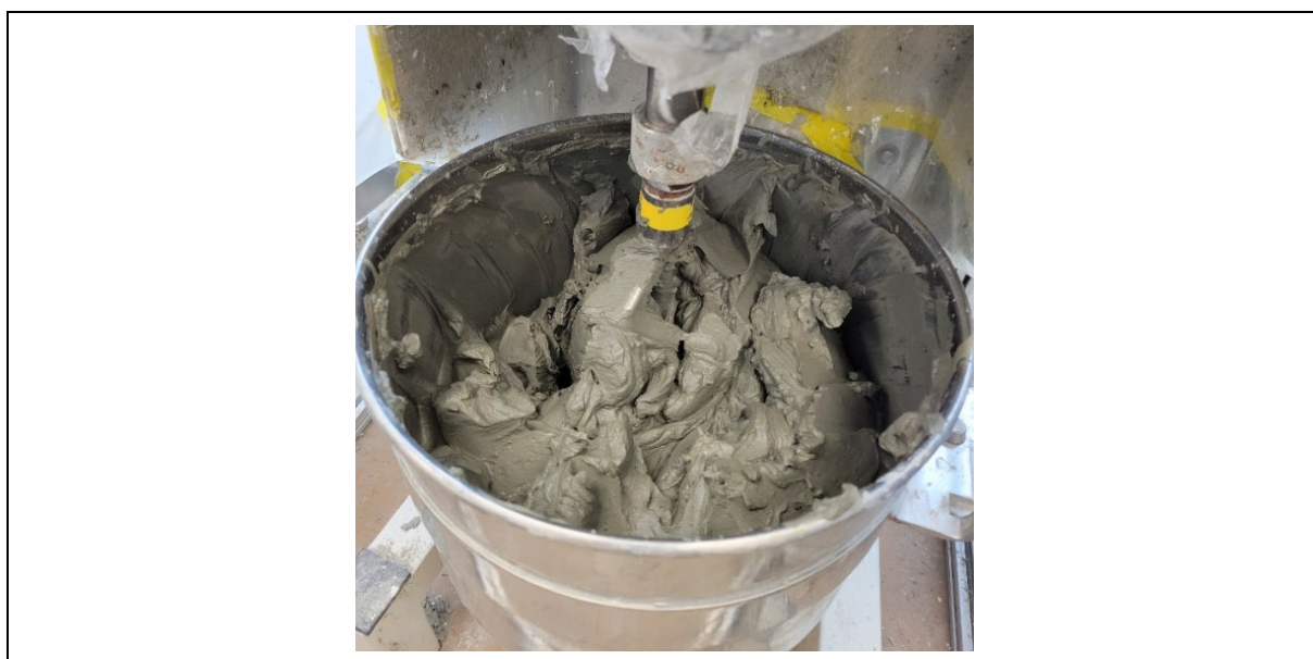
Figure 4.6 Soil-binder Mixture with Thoroughly Mixing
