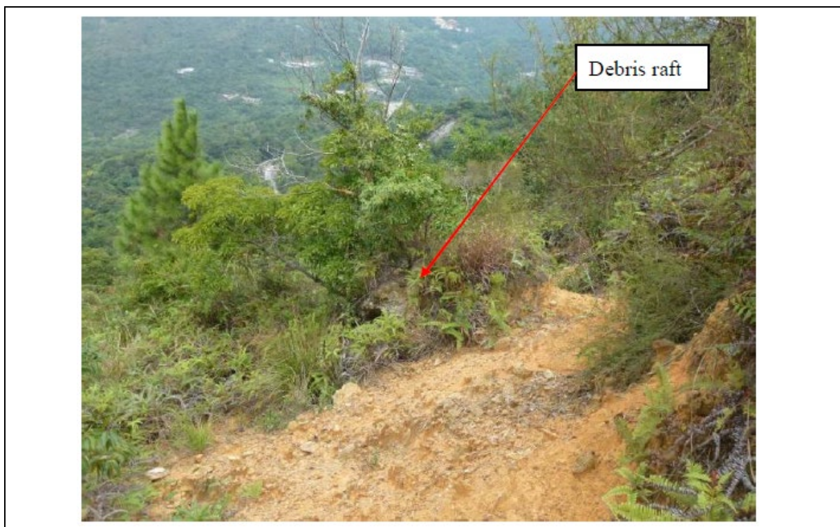
Plate D4.8 Displaced Intact Debris Raft on Recent Landslide ID No. 135 in Catchment KSR56A
