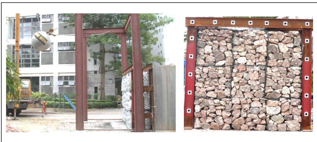
Figure B2 Impact Tests on Rigid Barrier with Rockfill Gabion Cushion (Lam, 2016)
