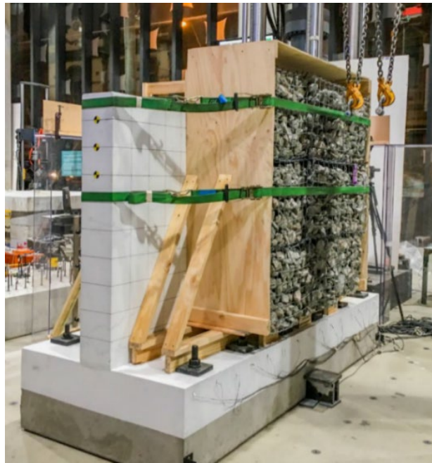
Figure 2.4 Overview of Rigid Barrier with Granite Gabions
