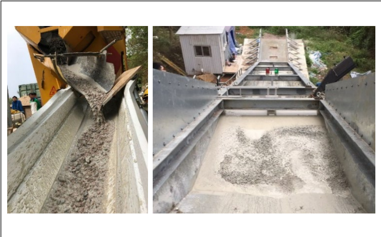
Figure 2.3 Mixing of Debris Materials by a Concrete Truck Mixer (Left) and Debris Stored at the Storage Container (Right)
