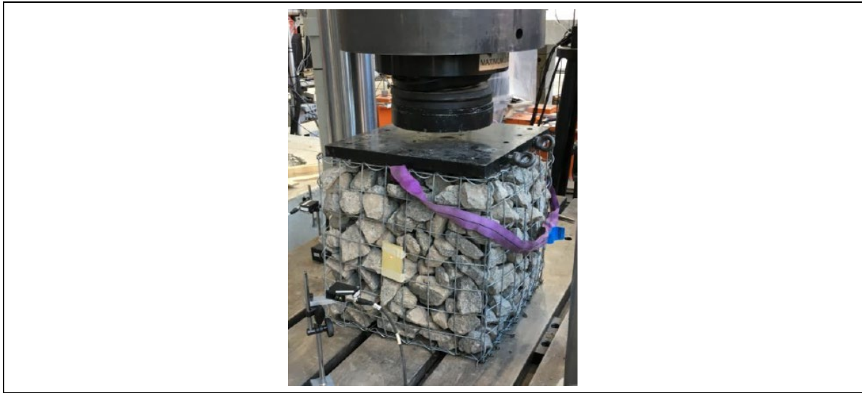
Figure B3 Uniaxial Compression Test on Specimen of Rockfill Gabion Cushion
