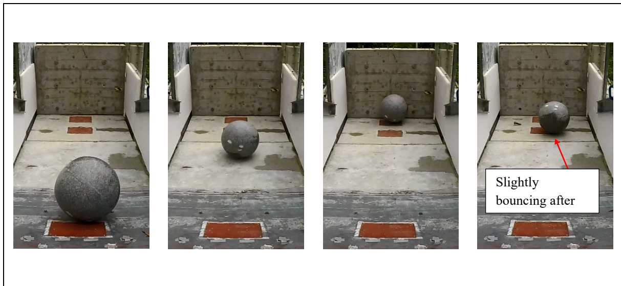
Figure 3.3 Snapshots of Test No. K5 Taken from High Speed Camera inside the Flume
