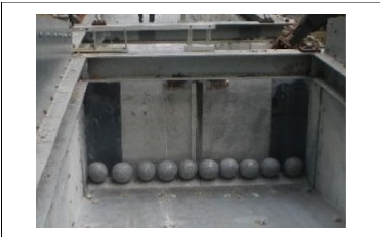
Figure 2.4 Ten Numbers of 200 mm Diameter Granitic Spheres for Simulation of Hard Inclusion in Test No. 2
