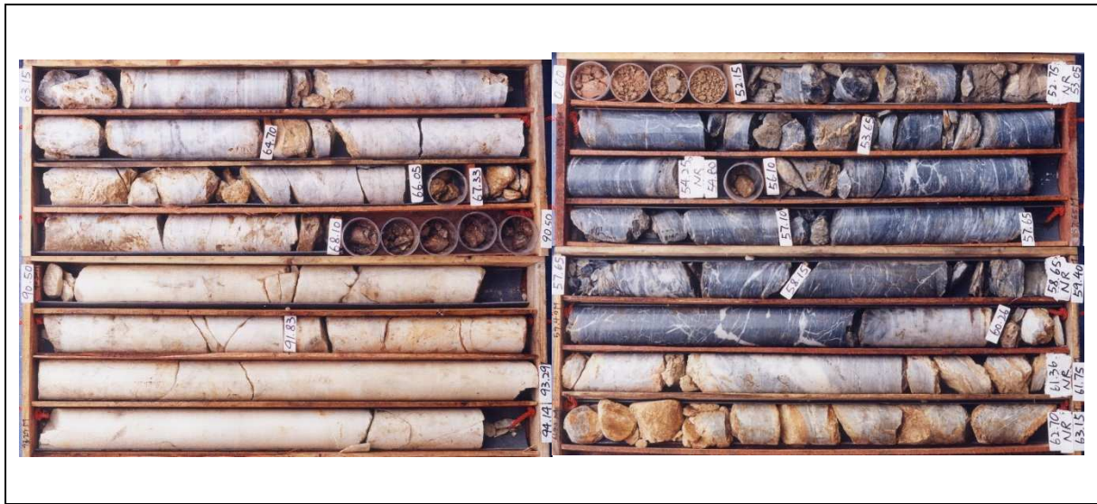
Figure 4.4 Gradational Contact between Long Ping and Ma Tin Members (Long Ping, GIU No. 35413/DH/647, Left: 0 - 63.15 m, Right: 63.15 - 94.14 m Depth)
