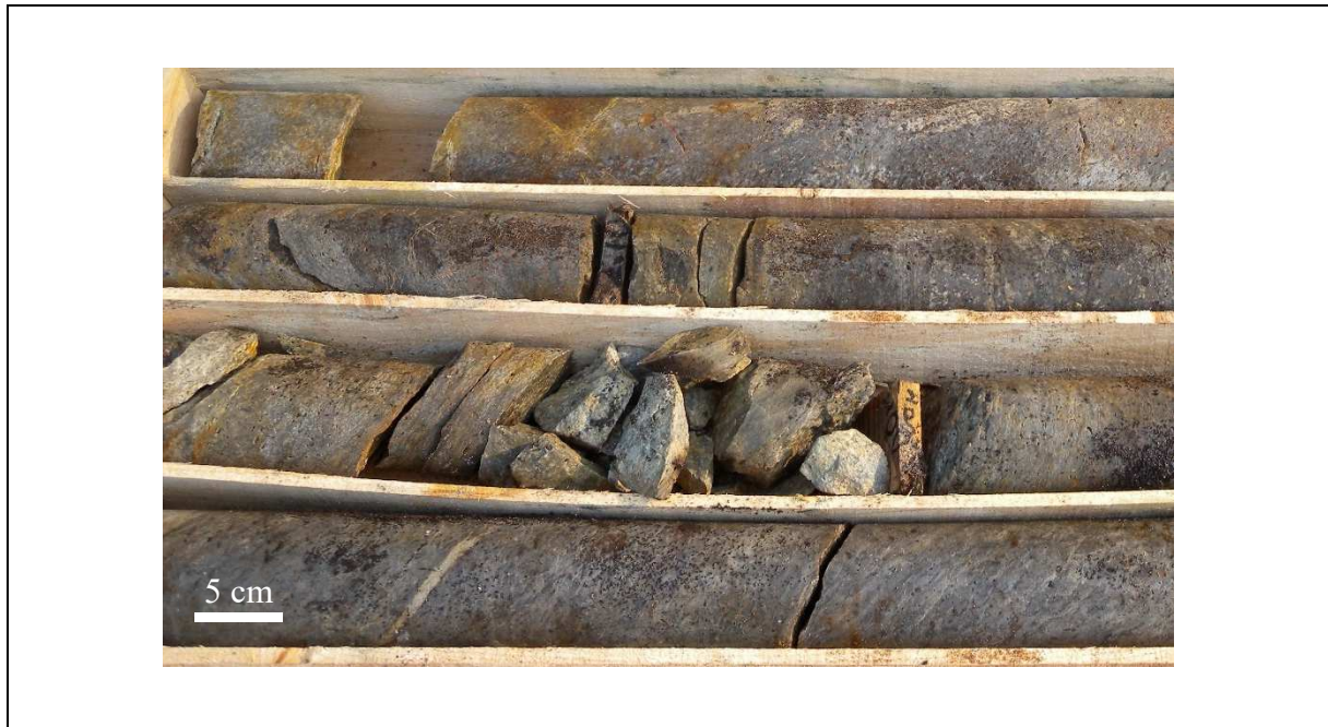
Figure 4.10 Intensely-silicified Mylonite (Near Tung Shing Lei, [8223 8344], Borehole No. DH56, 60.95 [Top Left] - 64.28 m [Bottom Right] Depth)
