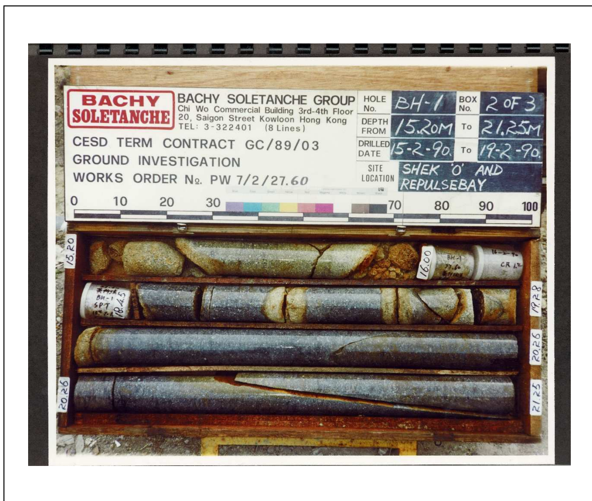
Figure 4.5 Coarse Ash Crystal Tuff in the Ap Lei Chau Formation, Based on BSG (1990)
