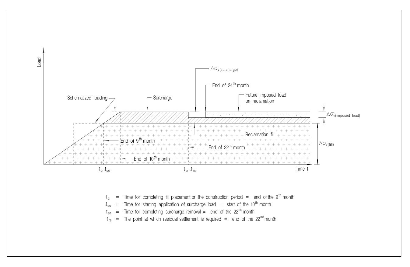
Figure D1 - Example 2: Loading Variations of the Reclamation
