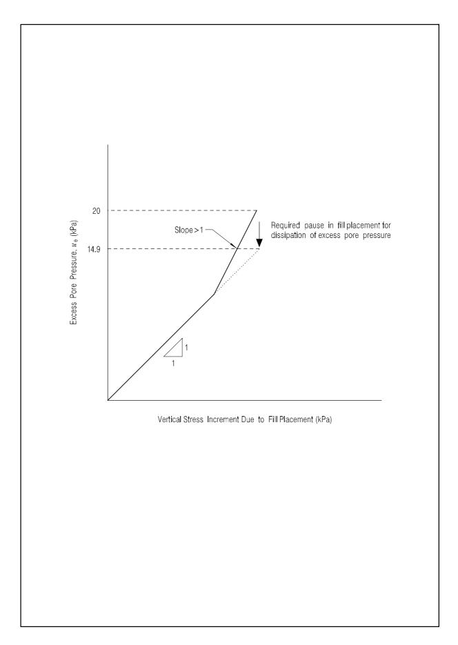
Figure D2 - Example 3: Pore Pressure Monitoring Data
